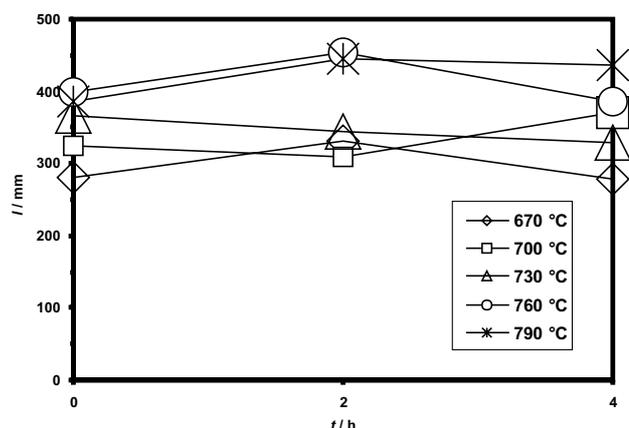
**Figure 3:** The castability (total length  $l$  of branches of experimental castings in mm) of quasi-ternary eutectic  $\text{AlZn}_7\text{Mg}_7\text{Cu}_1\text{Ni}_3\text{Si}_3$  (Be) alloy as the function of pouring temperature and holding time at pouring temperature
