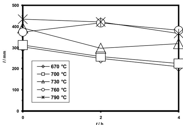
**Figure 4:** The castability (total length  $l$  of branches of experimental castings in mm) of  $AlSi_{10}$  (Be) alloy as the function of pouring temperature and holding time at pouring temperature
