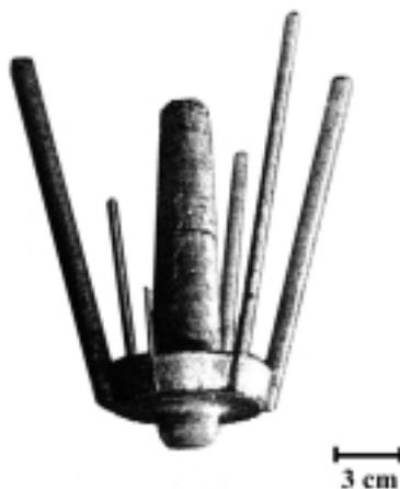
**Figure 1:** The casting of "sputnik" type used for the determination of the castability of alloys
