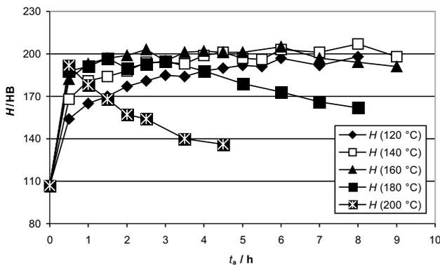
**Figure 6:** Age hardening curves of the the quasi-eutectic alloy  $\text{AlZn}_7\text{Mg}_7\text{Cu}_1\text{Ni}_3\text{Si}_3$  obtained after heating at  $520^\circ\text{C}$  (4 hours), water quenching and ageing at different temperatures
