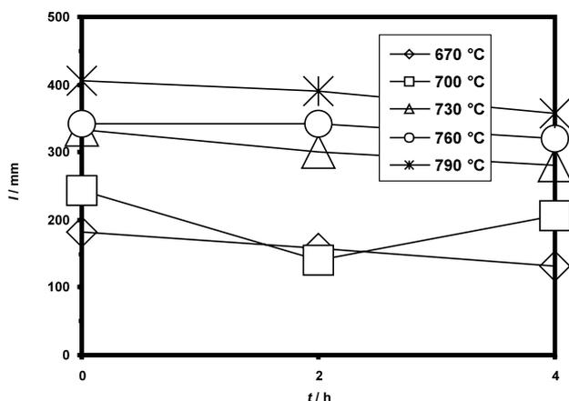
**Figure 5:** The castability (total length  $l$  of branches of experimental castings in mm) of  $AlZn_7Mg_2Cu_1$  (Be) alloy as the function of pouring temperature and holding time at pouring temperature
