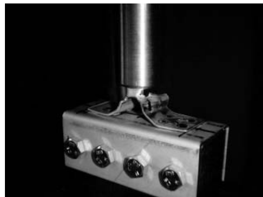
Figure 8: Static pulling test of holder
