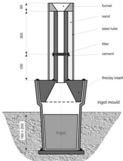
Figure 1: Design and placement of the ceramic filter
