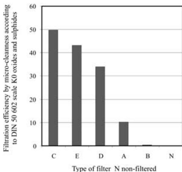
**Figure 7:** Filtration efficiency as micro-cleanliness according to DIN 50 602
