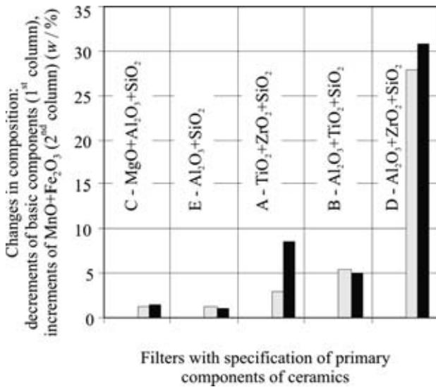
**Figure 2:** Decrements and increments of oxides in the coating of the filter capillaries
