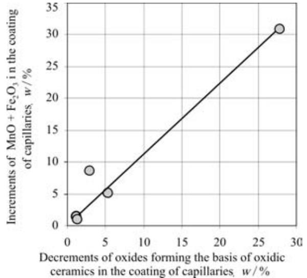
**Figure 3:** Relation between the decrements and increments of the oxides in the coating of the filter capillaries
