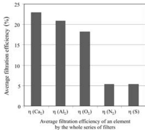
**Figure 4:** Filtration efficiency for the elements Ca, Al, O, N, S
