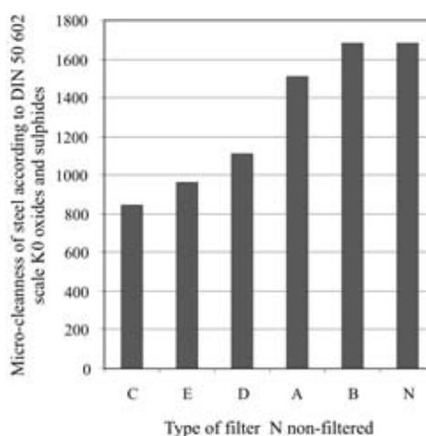
**Figure 6:** Micro-cleanliness of filtered steel according to DIN 50 602**Slika 6:** Mikročistota filtriranega jekla po DIN 50 602
