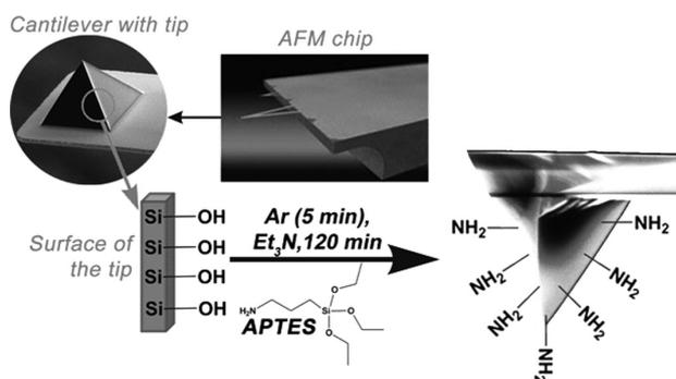
**Figure 1:** Preparation scheme for the amino functionalized AFM tips
