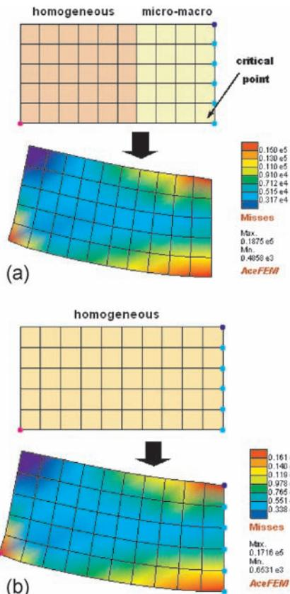
**Figure 3:** Macroscopic effective stress in micro-macro and homogenized problem, voided microstructure
