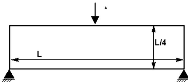
**Figure 2:** Three-point bending test
