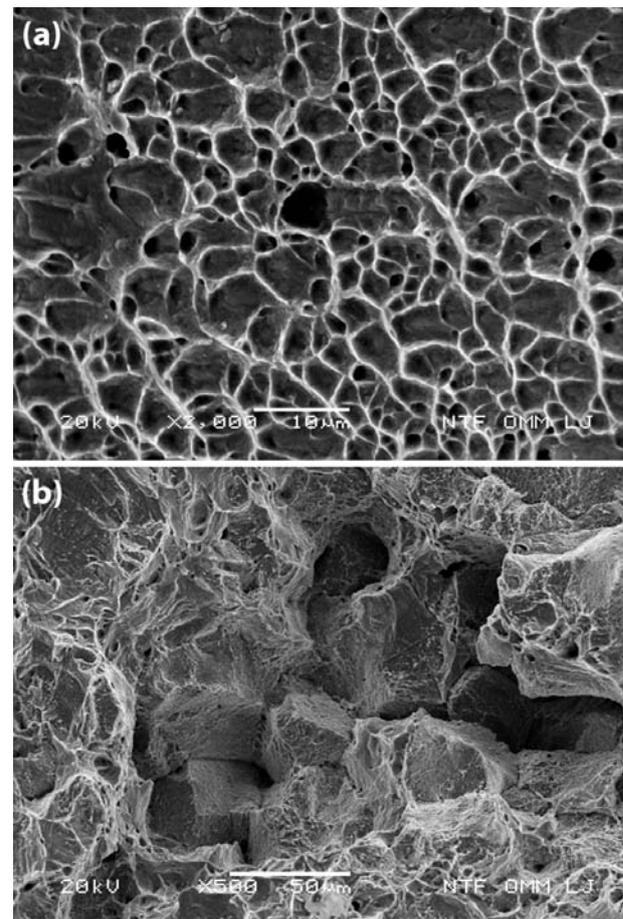
**Figure 3:** Fracture surface – SEM: a) room temperature and b) 750 °C
