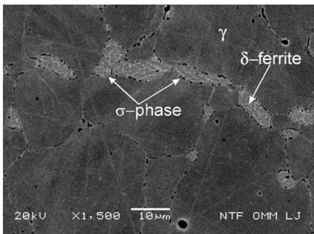
**Figure 2:** SEM microstructure samples tested at 750 °C
