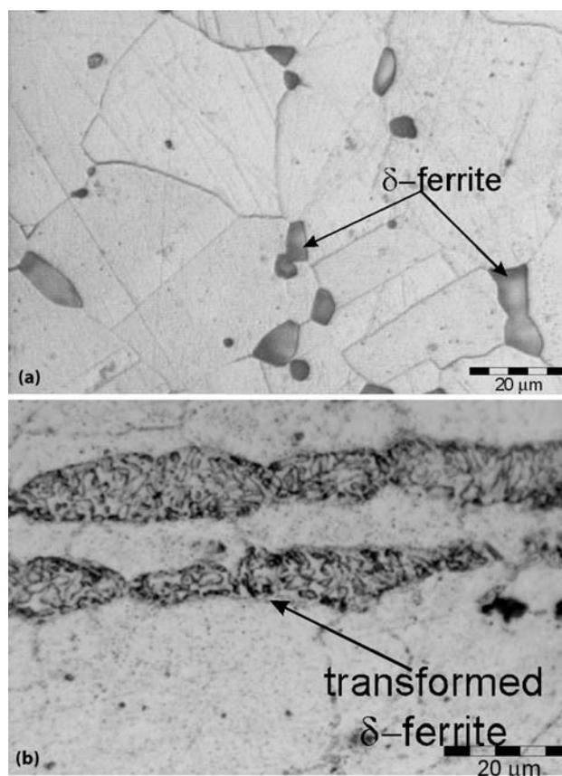
**Figure 1:** Microstructure of steel Nitronic 60 at: a) room temperature and b) 750 °C
