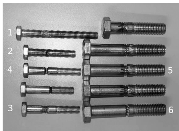
Figure 3: Different thrust screws. With small diameters we gain a compact design and with large diameters we gain more force. The design of a groove is crucial.
