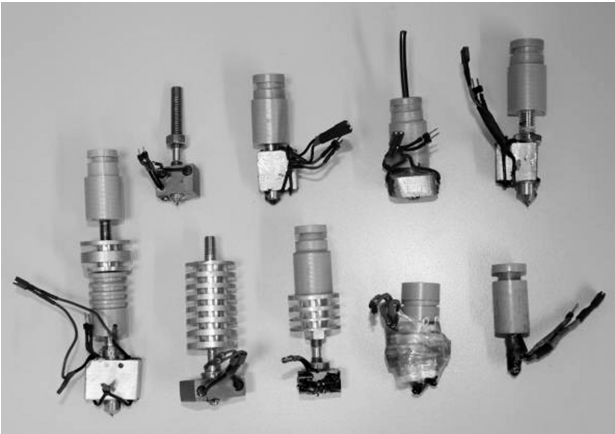
Figure 4: Different hot-end designs. Basically a hot end is assembled of a heater (a resistor), a nozzle, connection tubes and a thermal barrier (Teflon can be used, but PEEK is better).
