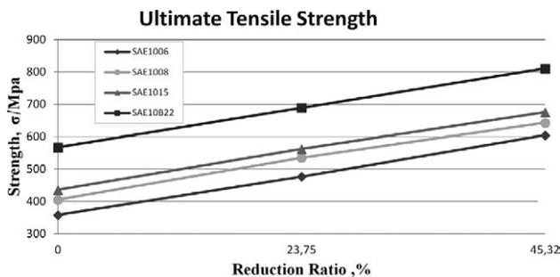
**Figure 13:** Variation in the ultimate-strength values for a rod and coil steel wire at a constant velocity (3.6 m/s) and different reduction ratios – different inlet diameters and constant outlet diameters (from  $\phi 5.50$  to  $\phi 4.81$  and from  $\phi 6.50$  to  $\phi 4.81$ )
