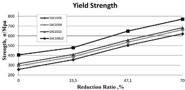
**Figure 9:** Variation in the yield-strength values for a rod and coil steel wire at a constant velocity and different reduction ratios (from  $\phi 5.50$  to  $\phi 4.81$ , to  $\phi 4.00$  and to  $\phi 3.01$ )
