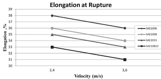
**Figure 17:** Variation in the elongation-at-rupture (%) values for a coil steel wire at a constant reduction ratio (from  $\phi 5.50$  to  $\phi 4.81$ ) and with different drawing velocities (3.6 m/s and 2.4 m/s)
