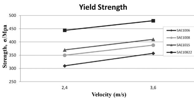
**Figure 15:** Variation in the yield-strength values for a coil steel wire at a constant reduction ratio (from  $\phi 5.50$  to  $\phi 4.81$ ) and with different drawing velocities (3.6 m/s and 2.4 m/s)
