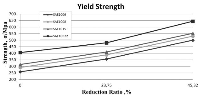
**Figure 12:** Variation in the yield-strength values for a rod and coil steel wire at a constant velocity (3.6 m/s) and different reduction ratios – different inlet diameters and constant outlet diameters (from  $\phi 5.50$  to  $\phi 4.81$  and from  $\phi 6.50$  to  $\phi 4.81$ )
