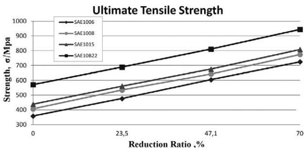
**Figure 10:** Variation in the ultimate-tensile-strength values for a rod and coil steel wire at a constant velocity and different reduction ratios (from  $\phi 5.50$  to  $\phi 4.81$ , to  $\phi 4.00$  and to  $\phi 3.01$ )
