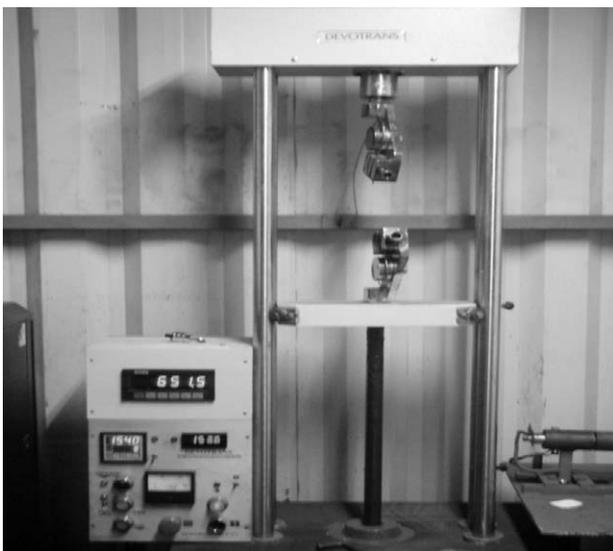
**Figure 3:** Tensile-test machine
