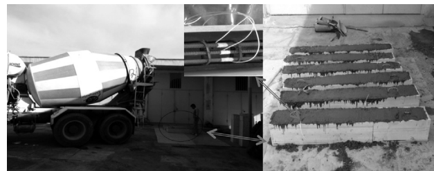
Figure 5: Reinforced concrete beams made by the authors (Gh.03) Slika 5: Armiranobetonski steber, ki so ga izdelali avtorji (Gh.03)
