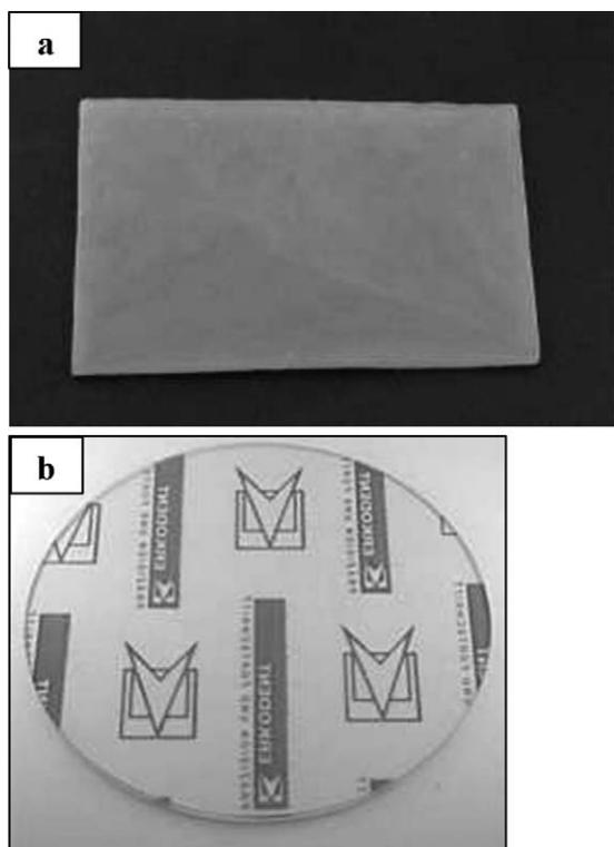
**Figure 1:** a) PMMA plate (Galenika, Serbia) and b) TPC plate (Erkodent, Germany)
