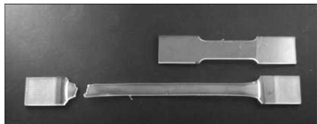
**Figure 4:** Elongation of the TPC tensile specimens before tensile testing and after the break
