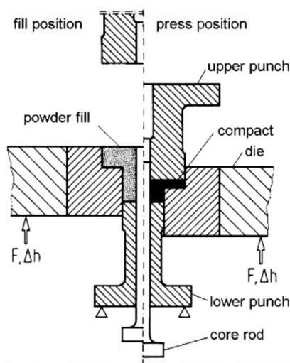
**Figure 7:** Schematic presentation of the cross-section of the tool for the uniaxial ADC of the double-height product<sup>5</sup>
