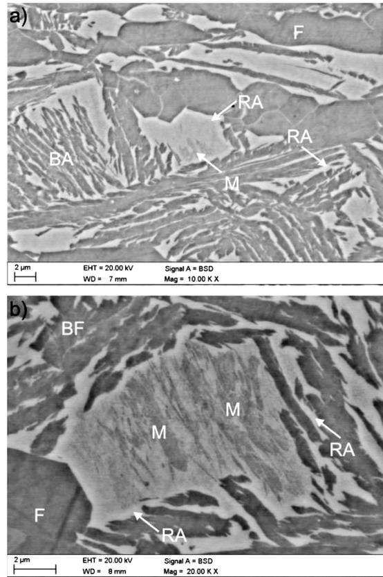
**Figure 2:** SEM micrographs showing strain-induced martensite in blocky grains of retained austenite at 5 % strain; magnifications of: a) 10000-times and b) 20000-times; F – ferrite, BA – bainitic-austenitic islands, RA – retained austenite, BF – bainitic ferrite, M – strain-induced martensite
