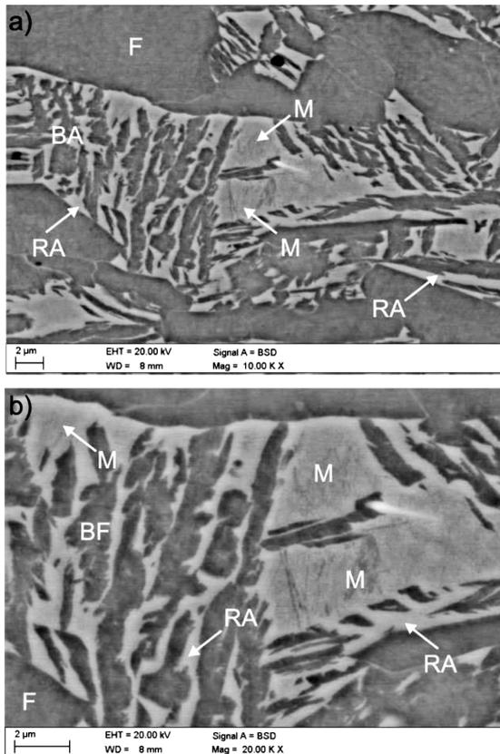
**Figure 4:** SEM micrographs showing strain-induced martensite in small blocky grains of retained austenite located in BA regions at 15 % strain: a) magnifications of 10000-times and b) 20000-times; F – ferrite, BA – bainitic-austenitic islands, RA – retained austenite, BF – bainitic ferrite, M – strain-induced martensite
