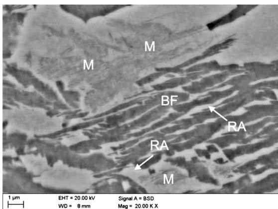
**Figure 5:** SEM micrograph showing strain-induced martensite in blocky grains of retained austenite and stable interlath retained austenite at rupture strain of 18.4 %; RA – retained austenite, BF – bainitic ferrite, M – strain-induced martensite
