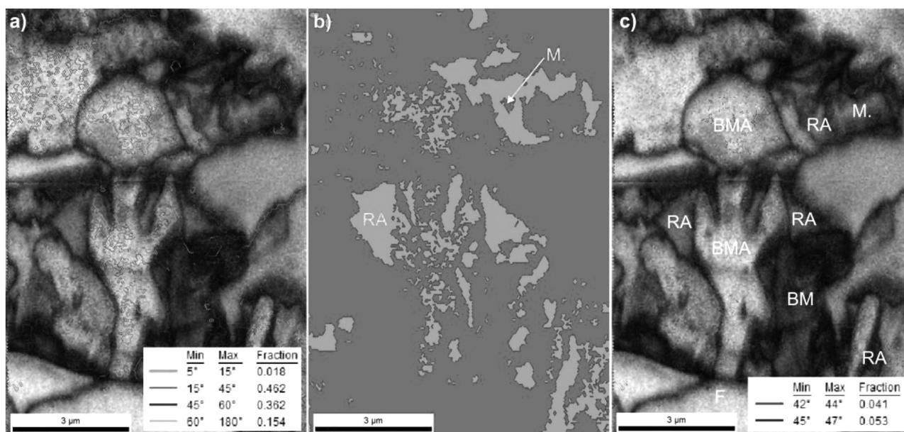
**Figure 3:** a) Image quality (IQ) map with misorientation angles, b) phase map showing retained austenite – RA regions, and c) IQ map with misorientation angles corresponding to the Kurdjumov-Sachs (42–44 °) and Nishiyama-Wasserman (45–47 °) relationships at 10 % strain; F – ferrite, BMA – bainitic-martensitic-austenitic constituents, RA – retained austenite, BM – bainitic-martensitic constituents, M – strain-induced martensite
