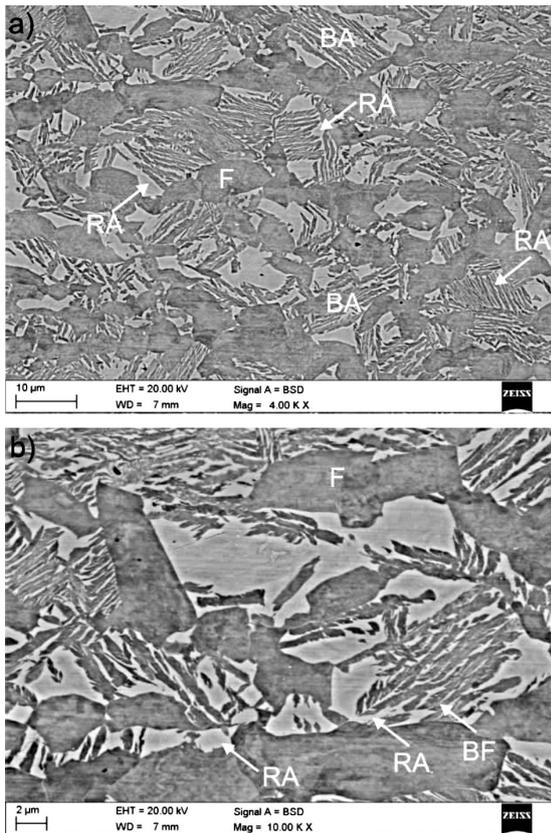
**Figure 1:** SEM micrographs of the: a) bainitic-ferritic steel containing blocky and interlath retained austenite after thermomechanical rolling, b) morphological details of the bainitic-austenitic (BA) islands; F – ferrite, BA – bainitic-austenitic islands, RA – retained austenite, BF – bainitic ferrite
