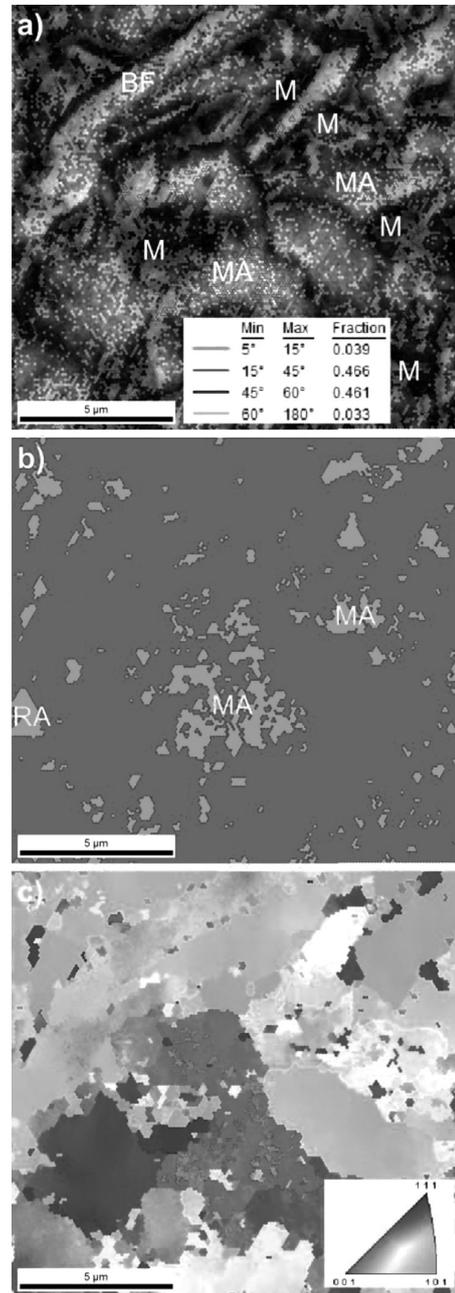
**Figure 6:** a) Image quality (IQ) map with misorientation angles, b) phase map showing retained austenite – RA regions, and c) inverse pole-figure map at rupture strain of 18.4 %; BF – bainitic ferrite, RA – retained austenite, MA – martensitic-austenitic constituents, M – martensite
