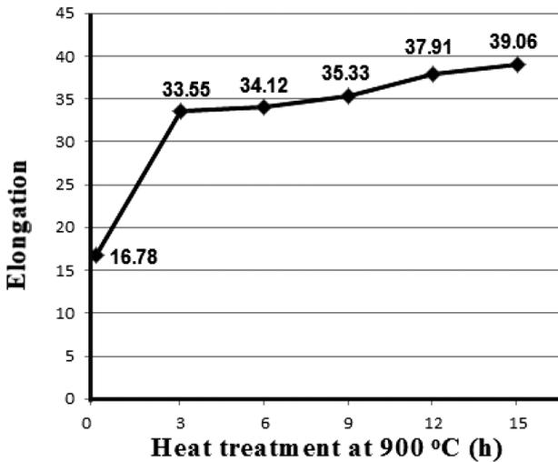
Figure 5: Heat-treatment effect on the elongation of free-cutting steel
