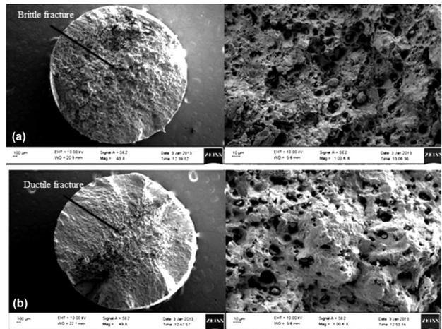
Figure 7: Macrostructures (49X) and microstructures (1000X) of fractured specimens: a) as received and b) heat treated at 900 °C for 15 h
