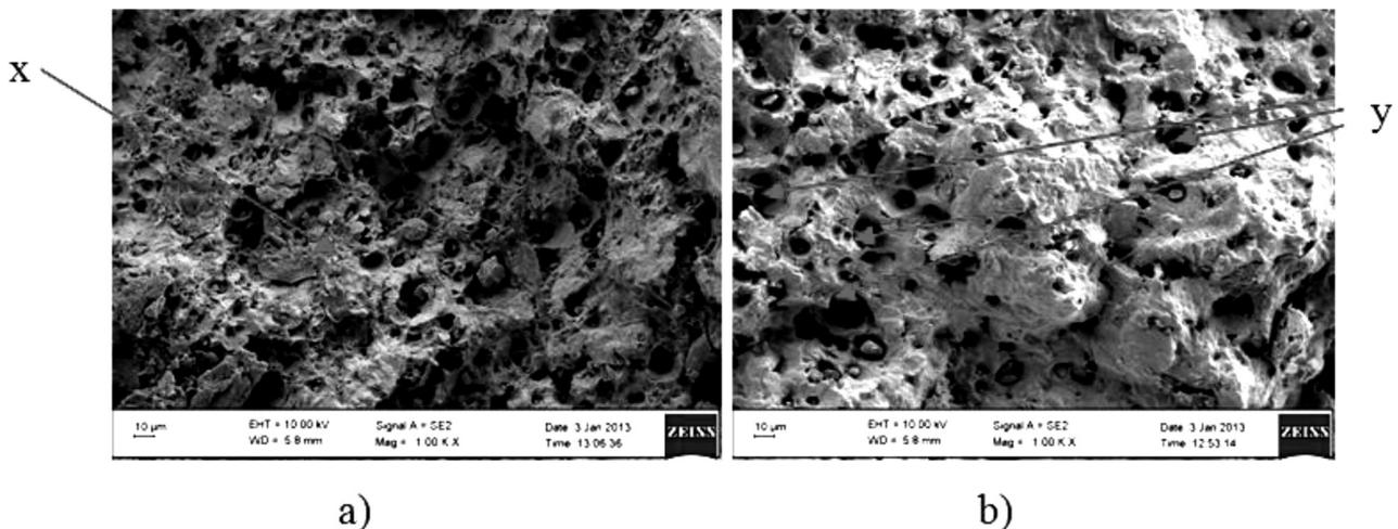
Figure 6: SEM images of fatigue-fractured surfaces of FCS: a) as received, b) heat treated at 900 °C for 15 h (x and y are voids)
