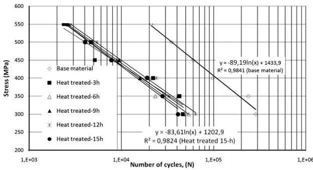
Figure 2: Effect of the heat exposure and time on the fatigue test results for FCS
