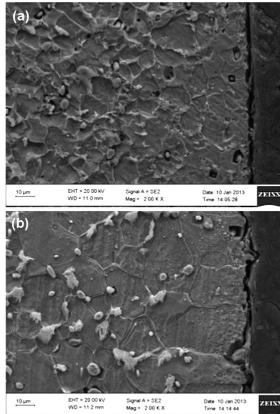
Figure 3: SEM images of grains: a) as received and b) heat treated at  $900 \text{ }^\circ\text{C}$  for 15 h
