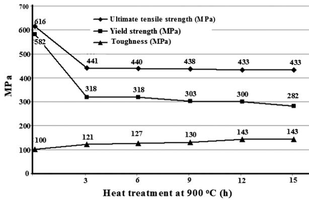
Figure 4: Effect of heat treatment on ultimate tensile strength ( $R_m$ ), yield strength ( $R_e$ ) and toughness of FCS
