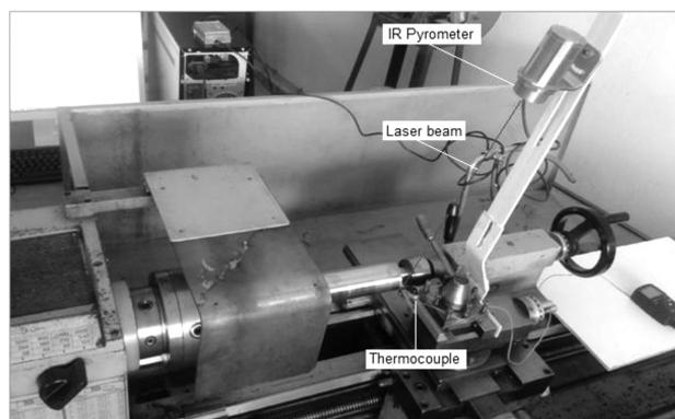
Figure 3: Thermocouple and IR pyrometer connections to the lathe
