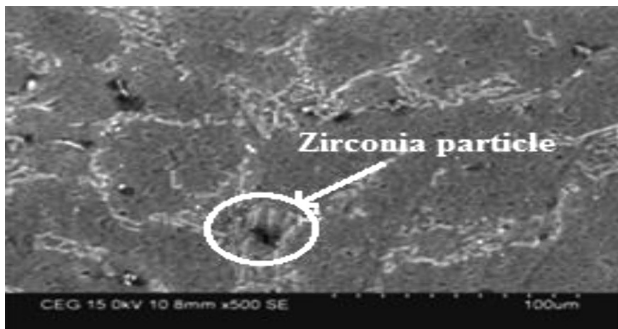
Figure 7: SEM image of LM6–6% of ZrO 2 Slika 7: SEM-posnetek LM6 – 6 % ZrO 2
