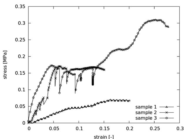
**Figure 3:** Stress-strain curves of the tested GG-BAG scaffolds
