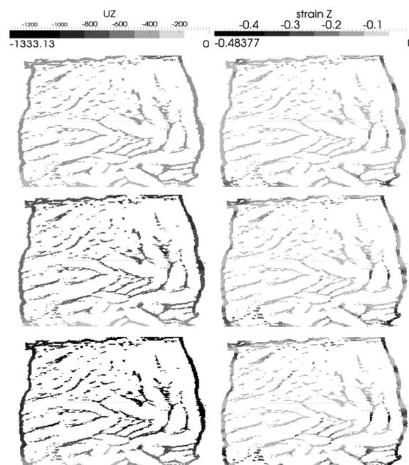
**Figure 6:** Displacement in z-direction ( $\mu\text{m}$ ) and Green-Lagrangian strain of the sample 1: 6 % overall deformation; 13 % overall deformation; 20 % overall deformation
