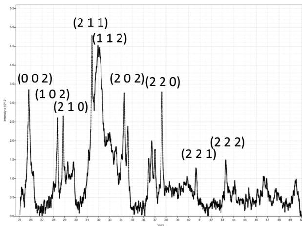
**Figure 2:** XRD diffractogram showing the HAP phases present in the coating
