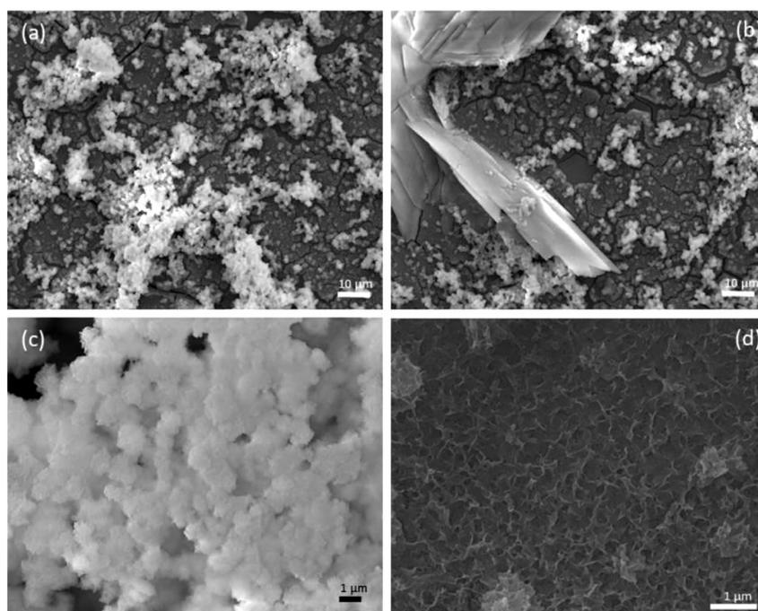
**Figure 1:** SEM images of surface morphology of HAP coating applied on the surface of NiTi alloy
