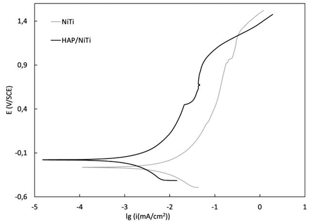
**Figure 3:** Potentiodynamic curves for HAP-coated NiTi alloy and bare NiTi substrate in a simulated physiological Hank's solution
