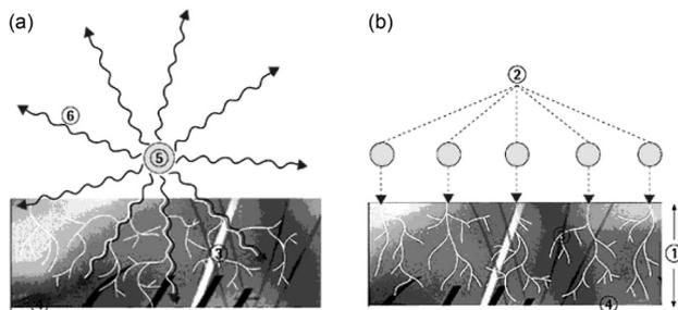
**Figure 1:** a) design of gamma rays and b) electron rays: 3 – secondary electrons, 4 – irradiated material, 5 – encapsulated Co – 60 radiation source, 6 – gamma rays. b) 1 – penetration depth of electrons, 2 – primary electrons, 3 – secondary electrons, 4 – irradiated material
