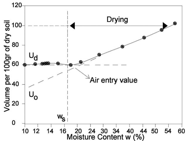
**Figure 2:** Shrinkage curve for Avanos solo clay
