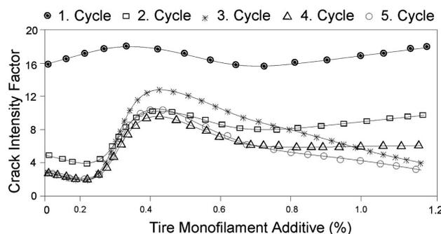
**Figure 7:** CIF for Avanos clay amended with tire monofilaments
