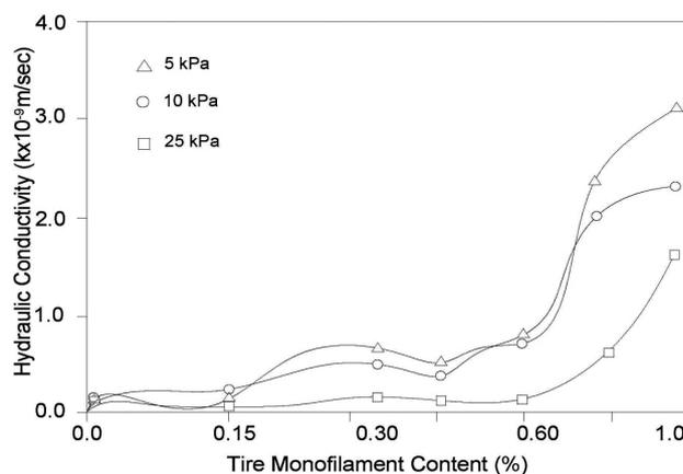
**Figure 6:** Hydraulic conductivity of mixed Avanos clay
