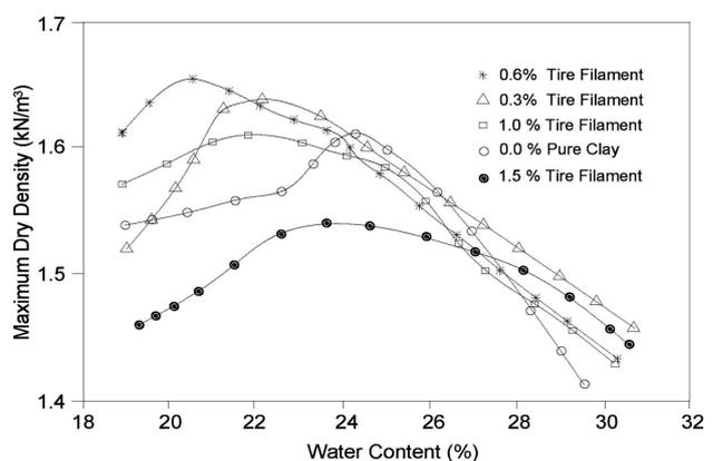
Figure 5: Compaction characteristics of mixed Avanos clay
