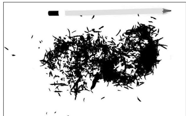
**Figure 3:** Tire monofilaments
