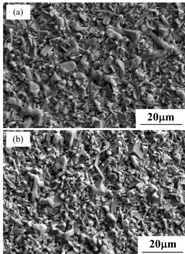
**Figure 2:** SEM of Ba<sub>2</sub>(Yb<sub>*x*</sub>Dy<sub>1-*x*</sub>)AlO<sub>5</sub> ( $x = 0, 0.3$ ) ceramics: a)  $x = 0$ , b)  $x = 0.3$
