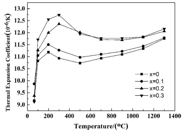
**Figure 4:** TECs of Ba<sub>2</sub>(Dy<sub>x</sub>Yb<sub>1-x</sub>)AlO<sub>5</sub> ( $x = 0\text{--}0.3$ ) ceramics
