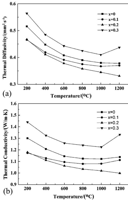
**Figure 3:** a) Thermal diffusivity and b) thermal conductivity versus temperature for Ba<sub>2</sub>(Dy<sub>x</sub>Yb<sub>1-x</sub>)AlO<sub>5</sub> ( $x = 0\text{--}0.3$ ) ceramics
