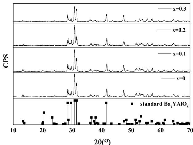
**Figure 1:** X-ray diffractograms of Ba<sub>2</sub>(Dy<sub>*x*</sub>Yb<sub>1-*x*</sub>)AlO<sub>5</sub> ( $x = 0\sim 0.3$ ) bulks
