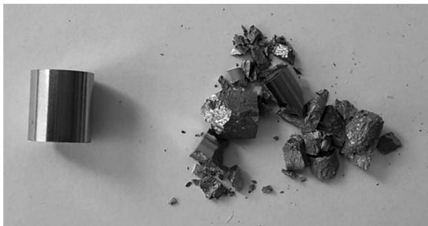
**Figure 9:** A test specimen of CVC NiTi rod before and after compressive test
