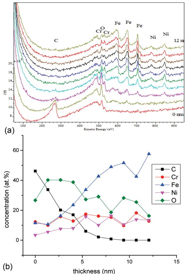
Figure 6: a) AES spectra, taken on retrieved metal mesh (AISI 316L), b) AES depth profile of the same metal mesh
