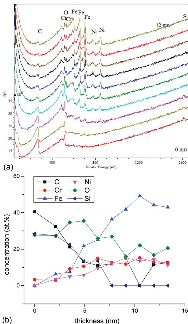
Figure 7: a) AES spectra, taken on new metal mesh (AISI 316L), b) AES depth profile of the same metal mesh
