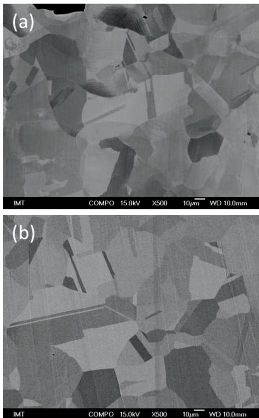
Figure 4: a) BE image of cross-section microstructures of retrieved and b) new metal mesh
