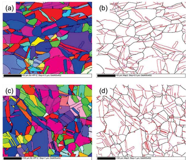
Figure 5: EBSD analysis of the metal mesh: a) orientation map of the new mesh, b) grain reconstruction of the new mesh, CSL Σ3 grain boundaries are shown in red, c) orientation map of the retrieved mesh, d) grain reconstruction of the new mesh, CSL Σ3 grain boundaries are shown in red
