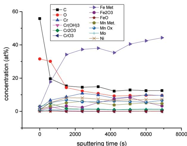
Figure 8: XPS depth profile of retrieved metal mesh (27 month)
