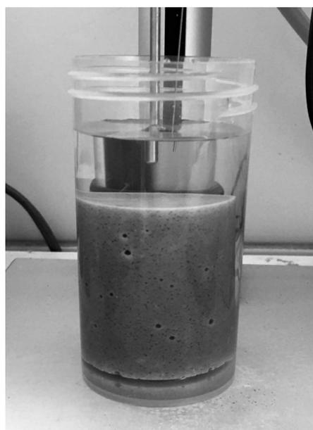
Figure 1: Dynamic surface-tension measurement
