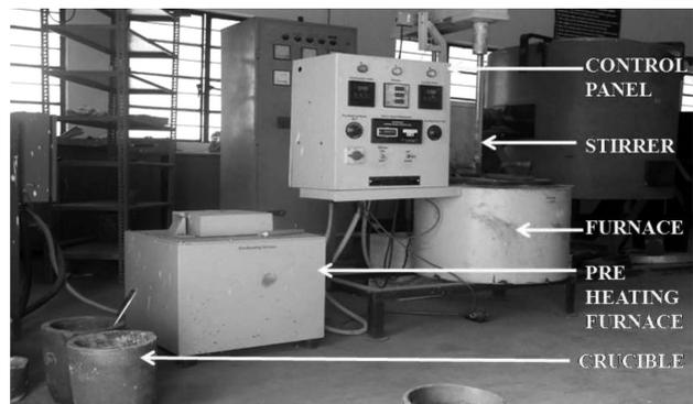
**Figure 2:** Experimental setup for stir casting
