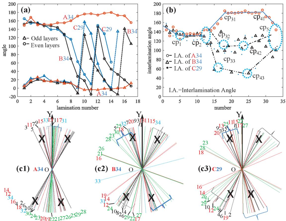
**Figure 2:** Fiber-lamination methods in three different parts of the *O. Rhinoceros* horn. a) Arrangement of the odd and even numbered layers, b) the intersection angle of the fibers between two adjacent layers, c) schematic line diagrams of the fiber orientation. The fibers (orientations) marked with X and the brace in the figure are the ones forming an X- or Y-shaped distribution. The data for the fiber lamination were reported by Zelazny and Neville.<sup>16</sup>
