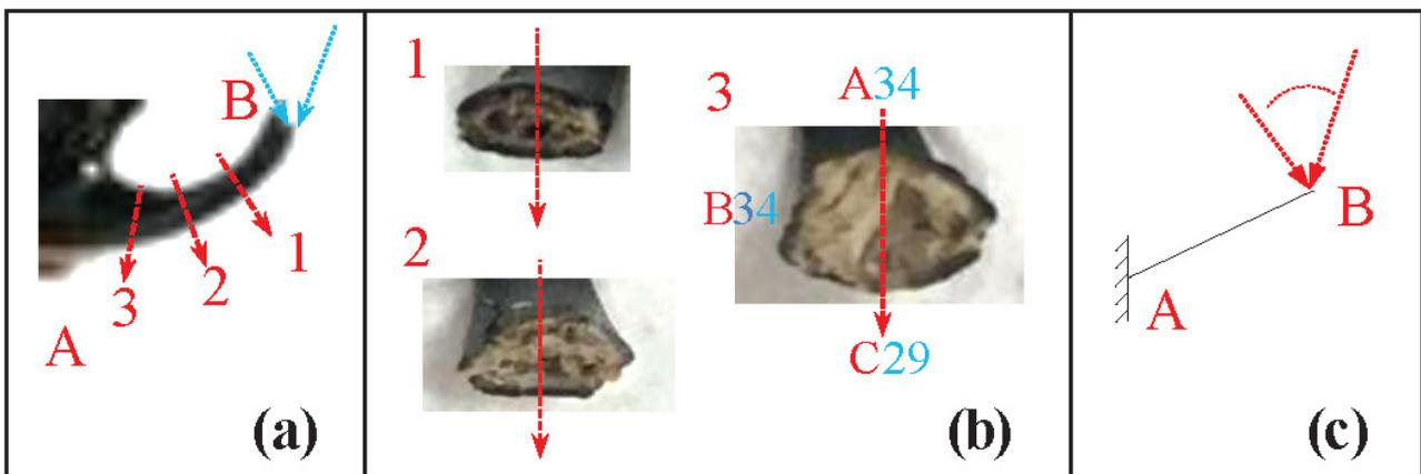
**Figure 3:** Photographs of *O. Rhinoceros* horn. a) Horn, b) cross-sections, and c) the schematic diagrams of the simplified mechanical model
