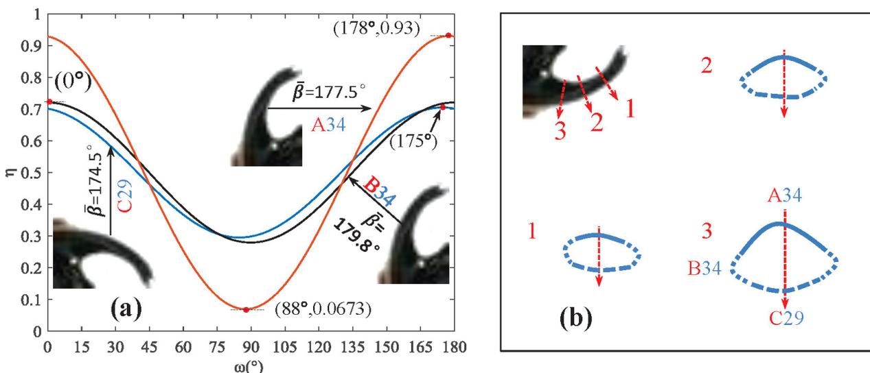
Figure 5: a) Plots of the average fiber orientation angles in the *O. Rhinoceros* horn and b) a schematic diagram of the three parts of each cross-section
