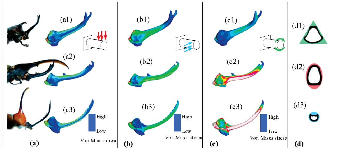
**Figure 4:** Von Mises stress distributions of the horn of *T. Dichotomus*, *D. Hercules* and *G. Porteris* under different directional forces. a) Vertical force, b) horizontal force, c) torsion and d) schematic diagrams of the cross-sections of the three beetles' horns. The data were reported by McCullough, Tobalske, and Emlen. (Reproduced from <sup>5</sup>, with permission from [PNAS])
