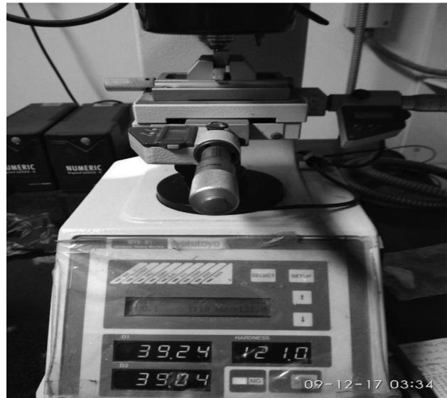
**Figure 3:** MITUTOYO microhardness tester
