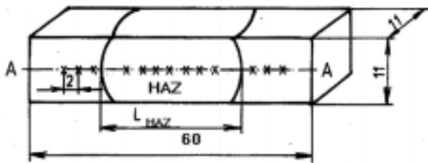
**Figure 5:** Simulated sample and positions (x) for hardness measurement
