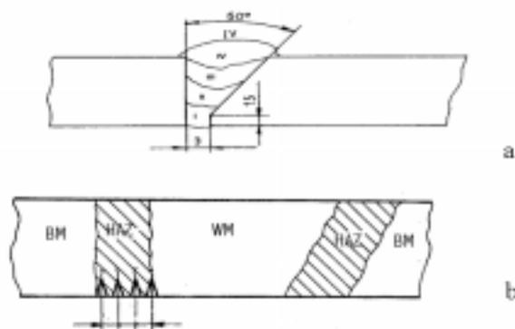
Figure 4: Steel A joint obtained by four passes manual welding arc (a) and crack tip position in the heat-affected-zone (b)
