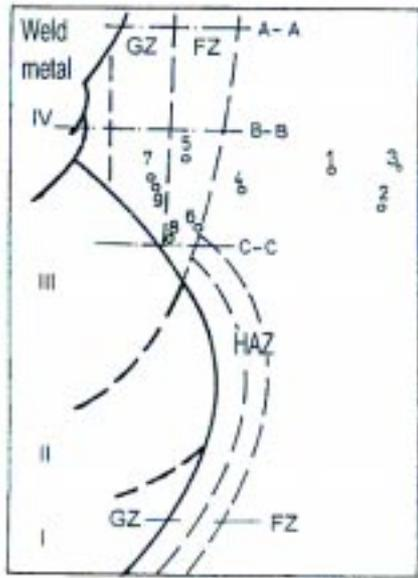
**Figure 7:** Crack tip locations for specimens 1 to 9 in different HAZ regions of individual welding runs (I to IV) in the welded joint of steel B (compare Table 6)
