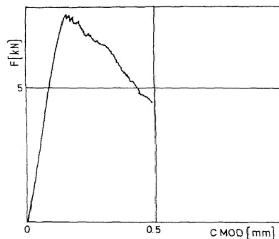
**Figure 2:** Load  $F$  vs. crack mouth opening displacement CMOD for brittle fracture of the specimen tested at  $-30^\circ\text{C}$
