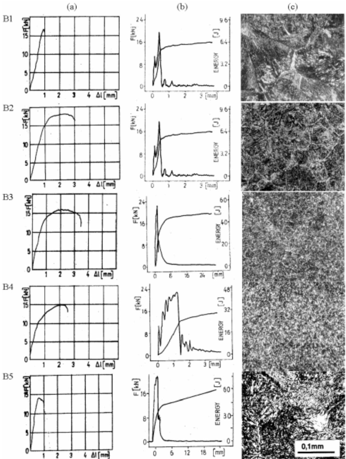
**Figure 6:** Dependences obtained by tensile tests and instrumented impact tests with corresponding microstructures of samples of steel B, simulated at different temperatures (B1 - 1350°C, B2 - 1100°C, B3 - 950°C, B4 - 850°C, B5 - 1350°C /750°C)
