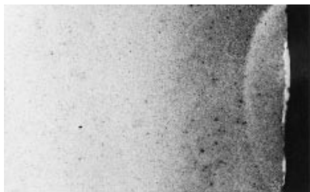
Slika 8: Radialni prerez skozi poškodbo na batu hidravličnega ventila Figure 8: Radial cross-section through the damage on the piston of a hydraulic valve
