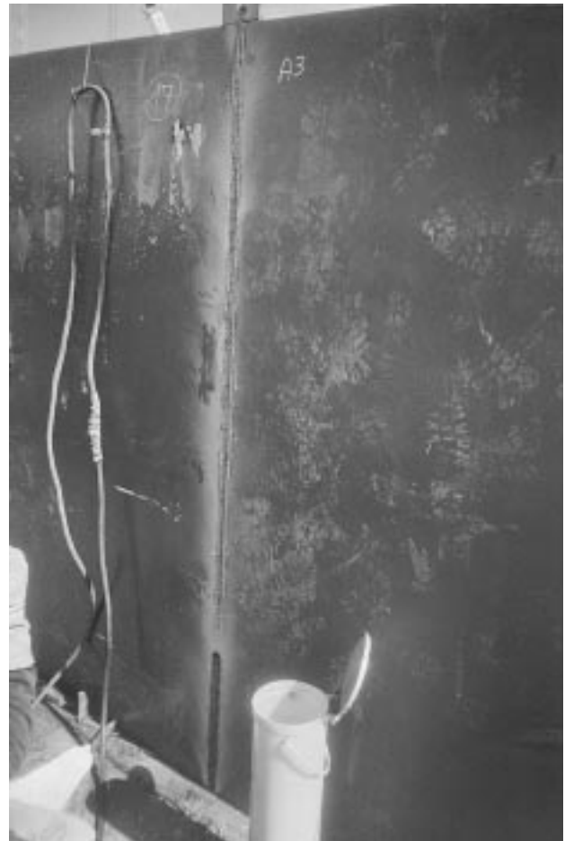
Slika 6: Vertikalni zvar dveh pločevin Figure 6: Vertical welding joint of two plates
