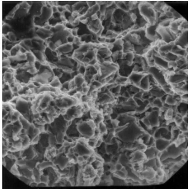
**Figure 9:** Edge of sample, Al/SiC compo-site, magnification: 500 x
