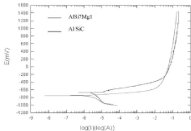
**Figure 4:** Curves of anode potentiodynamic polarization for the extruded Al/SiC MMC and the AlSi7Mg1 alloy in 3.5% water solution of NaCl
