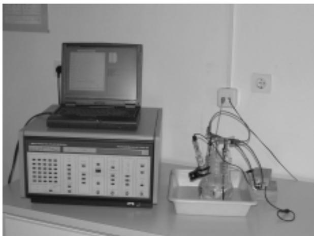
**Figure 1:** Electro-chemically-based determination of corrosion resistance using EG-G PAR potentiostat 273 and Softcorr-352 software (Corrosion Lab, Institute of Metals and Technology, Ljubljana, Slovenia)
