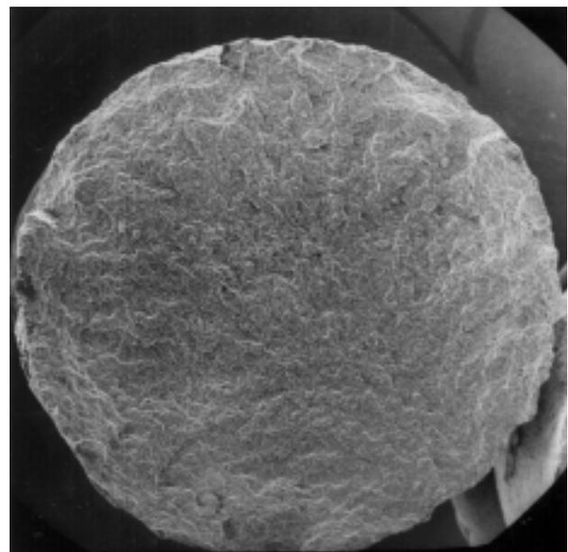
**Figure 6:** General corrosion in outer zone, AlSi7Mg1 alloy, mag.: 10 x
