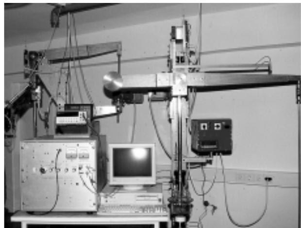
**Figure 2:** Laboratory equipment for anode and cathode electrochemical polarization of statically loaded samples
