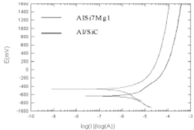
**Figure 3:** Curves of anode potentiodynamic polarization for the extruded Al/SiC MMC and the AlSi7Mg1 alloy in distilled water
