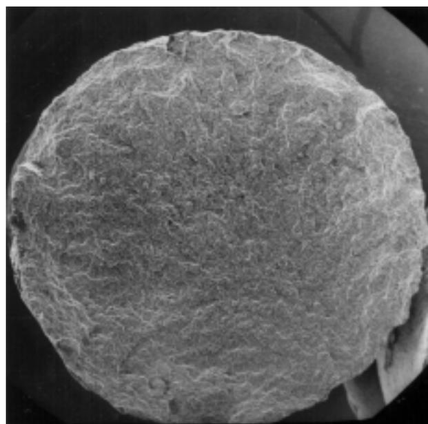
**Figure 6:** General corrosion in outer zone, AlSi7Mg1 alloy, mag.: 10 x
