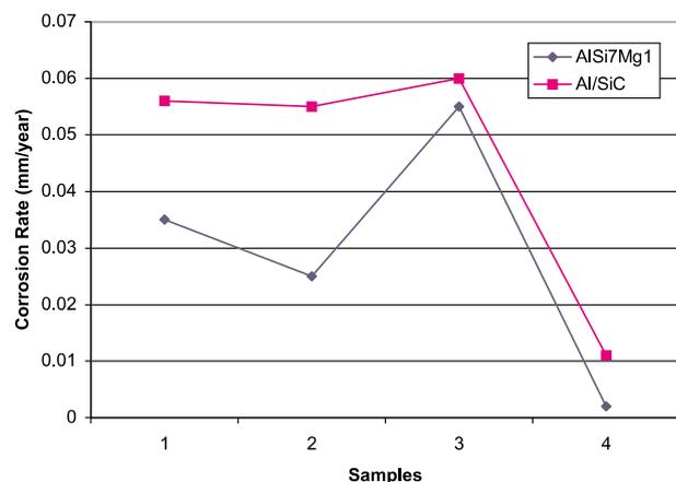
**Figure 5:** The comparison of corrosion rates for the Al/SiC composite and the AlSi7Mg1 alloy: **1)** as-extruded alloy in distilled water, **2)** heat-treated alloy in distilled water, **3)** as-extruded alloy in 3.5% water solution of NaCl, **4)** heat-treated alloy in 3.5% water solution of NaCl
