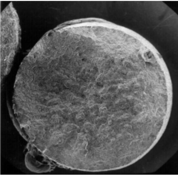
**Figure 7:** General corrosion in outer zone, Al/SiC composite, mag.: 10 x
