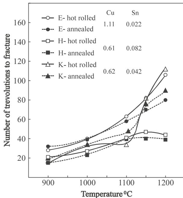
**Figure 13:** Number of revolutions to fracture in dependence on temperatures for the E, H and K steels in annealed and as hot rolled conditions
