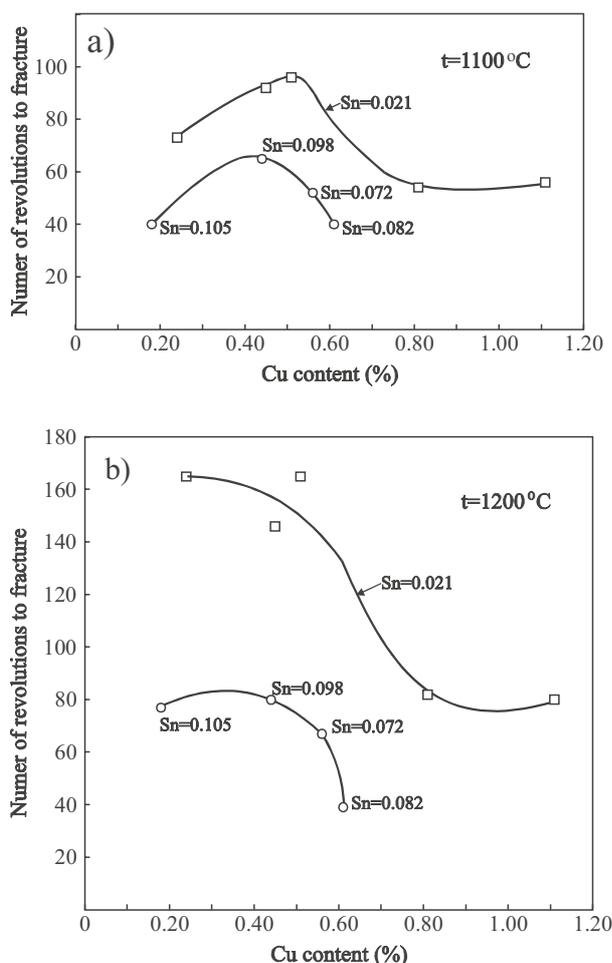
**Figure 12:** Number of revolutions to fracture by different copper and tin contents at different test temperature: a) 1100 °C; b) 1200 °C
