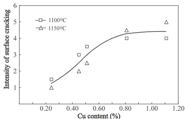
**Figure 2:** Effect of Cu content on surface shortness intensity at critical temperatures 1100-1150 °C
