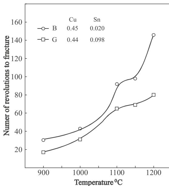
**Figure 11:** Number of revolutions to fracture in dependence on the temperature in steels B and G with identical content of copper and different content of tin
