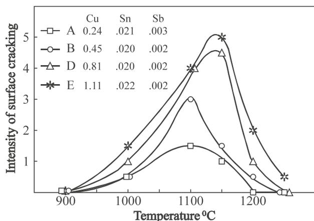
**Figure 1:** Intensity of surface cracking in dependance on heating temperature for the A, B, D, and E steels with different content of Cu and the constant content of Sn and Sb
