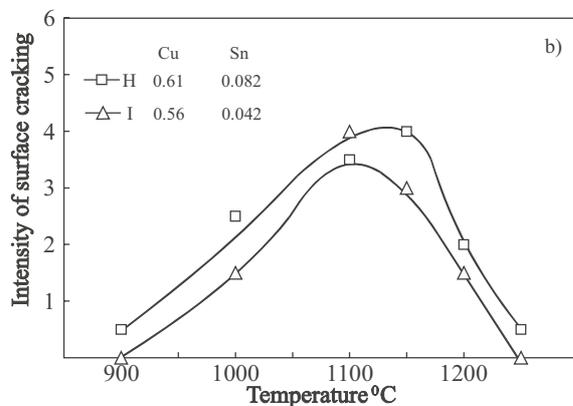
**Figure 6:** Intensity of surface cracking as function of temperature in: (a) B, G and (b) H, I steels
