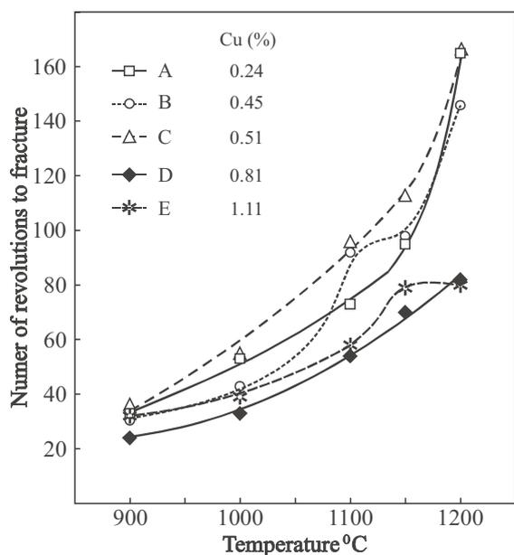
**Figure 10:** Number of revolutions to fracture in dependence test temperature for the A - E steels with different copper contents
