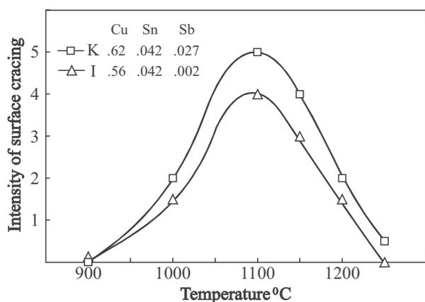
**Figure 9:** Surface crack intensity changes in function of temperature for I and K steels
