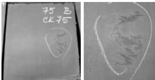
Slika 3: Notranje razpoke na lužilnih probah Figure 3: Internal cracks on a pickled specimen
