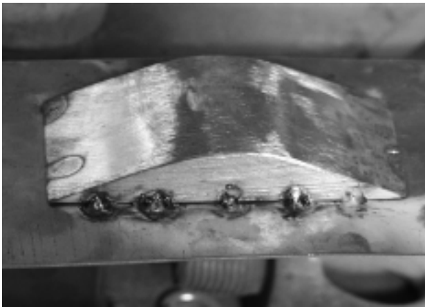
Slika 8: Zagozda za preskus deformiranja žile Figure 8: Wedge for the testing of the strand deformation
