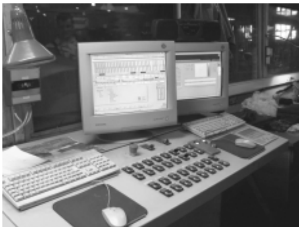
Slika 2: Nadzorni pult peči Allino – Simulacijski model ogrevanja gredic v realnem času ALLINOSIM3D (desni monitor) Figure 2: The command desk of the Allino-furnace – The real-time simulation model of the billet-reheating process ALLINOSIM3D (right monitor)
