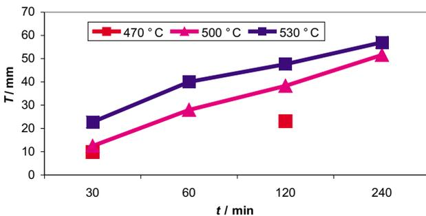
**Figure 6:** Thickness of the nitrided region as a function of temperature and dwell time
