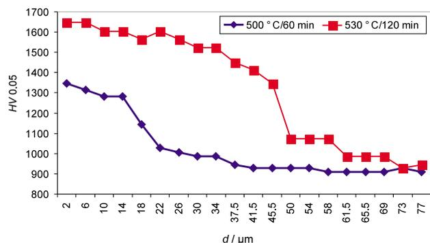
**Figure 12:** Microhardness depth profiles for various nitriding conditions
