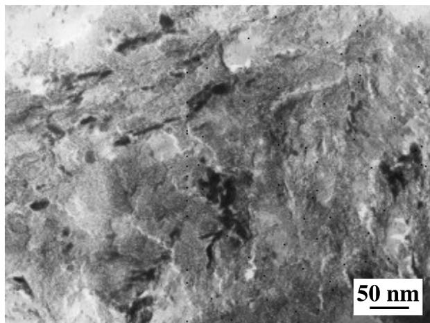
**Figure 10:** TEM micrograph of the plate-like nitrides in the near-surface region, collodion replica
