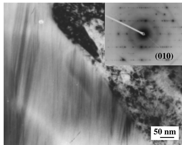
**Figure 8:** TEM micrograph of a coarse  $M_7(C,N)_3$  particle
