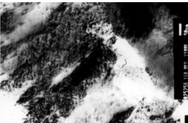
**Figure 2:** TEM micrograph of the matrix, dislocated martensite, thin foil.
