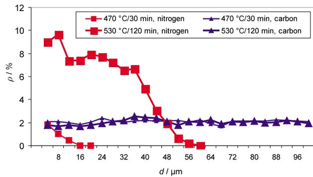
**Figure 11:** Nitrogen- and carbon-concentration depth profiles for the specimens processed at 470 °C for 30 min and 530 °C for 120 min
