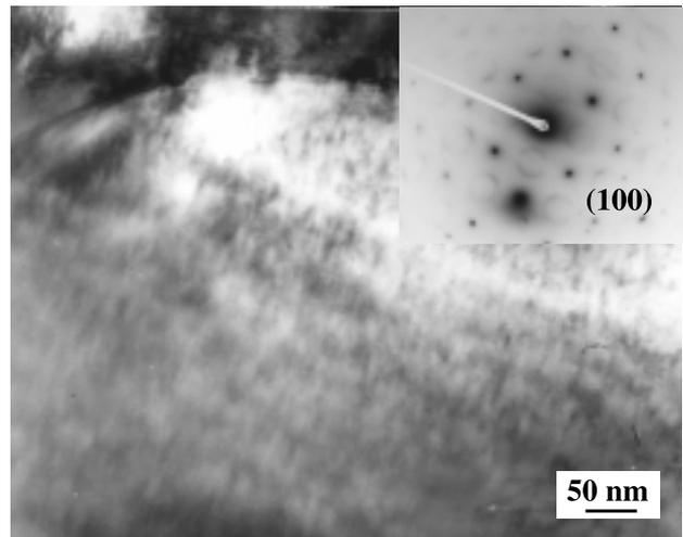
**Figure 7:** TEM micrograph of a coarse M(C,N) particle
