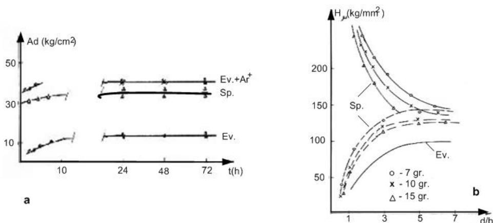
**Figure 7:** Adhesion and microhardness of dental gold thin films on acrylate substrate: a) adhesion vs. aging time of evaporated (•), and evaporated and then Ar<sup>+</sup> bombarded (x) thin gold films; b) microhardness vs. d/h for different loads on glass (solid lines) and on acrylate (broken lines).
