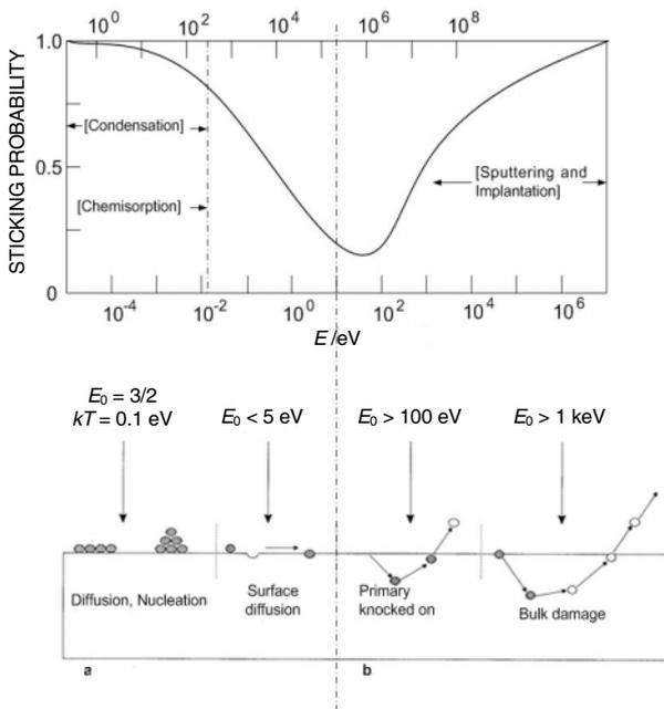
**Figure 1:** Illustration of the interaction processes as a function of ion-beam energy: a) low-energy ions and b) collision cascade.
