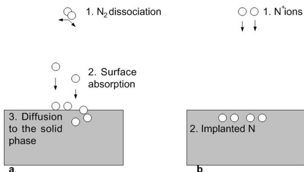
**Figure 3:** The kinetic path for a) thermally activated and b) ion-beam activated nitriding.
