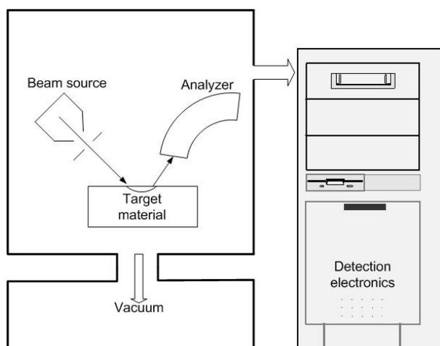
**Figure 2:** Schematic illustration of the beam technique for structural and compositional analyses.
