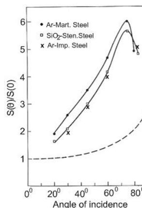
**Figure 5:** Variation of sputtering yield of stainless steel as a function of the angle of incidence:  $\text{Ar}^+$  on martensitic steel ( $\bullet$ ), silica on austenitic steel ( $\square$ )  $\text{Ar}^+$  on implanted steel ( $\times$ ); the dashed line indicates the theoretical prediction.
