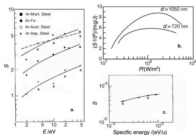
**Figure 4:** Experimental sputtering yields data vs. incident energy of the: a)  $\text{Ar}^+$ -ion beam, b) laser beam and c) mechanical-particles beam
