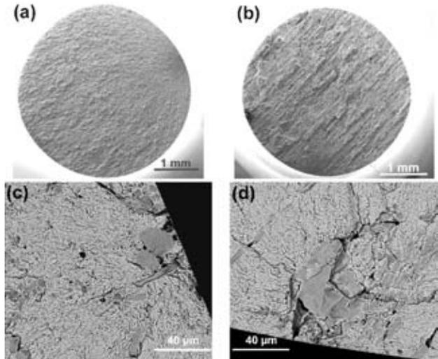
Figure 2: Fracture surface overviews of ASIS D2 type wrought cold work tool steel: (a) K110LL, (b) K110TT; primary carbide clusters to be crack origins of (c) K110LL and (d) K110TT specimens.
