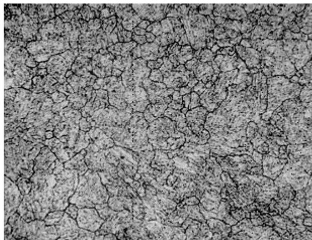
**Figure 1:** Inacceptable dies microstructure
