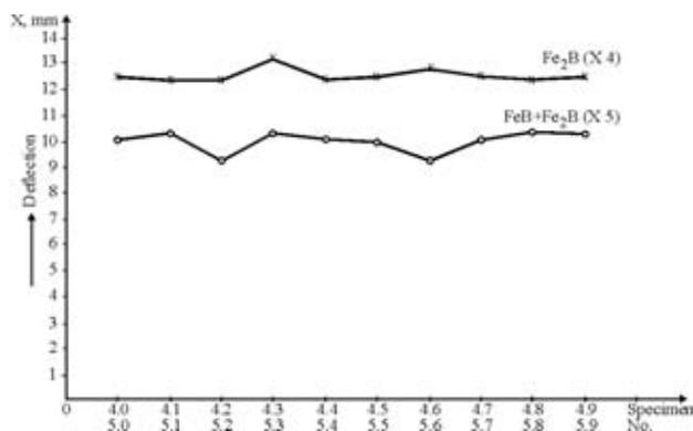
Figure 3: Results boride layers ductility examination by bending
