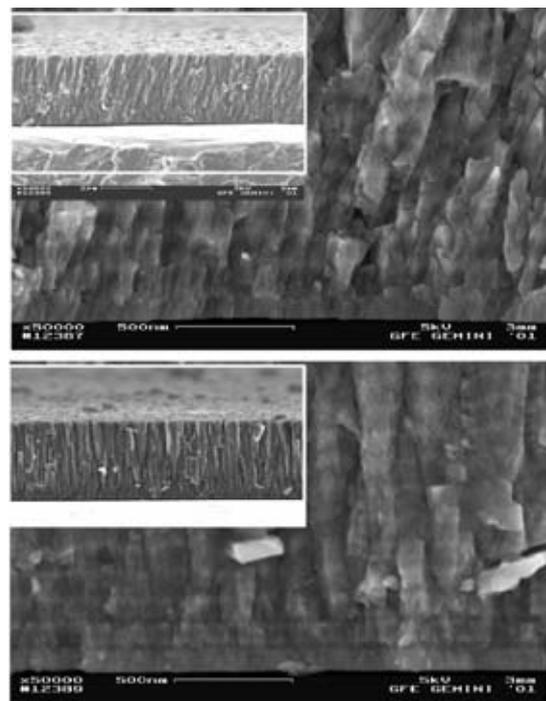
Figure 2. SEM micrographs of coatings, increasing of sputtering power versus thickness a. 500W b. 1000W
