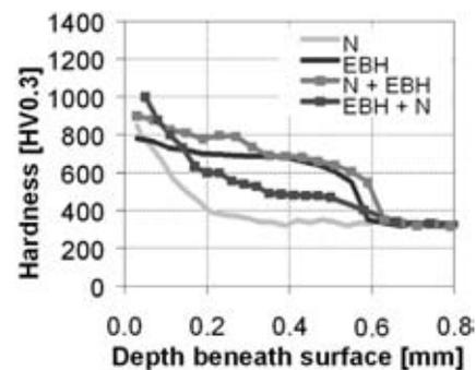
Figure 2: Hardness depth profiles of the combination of N and EBH
