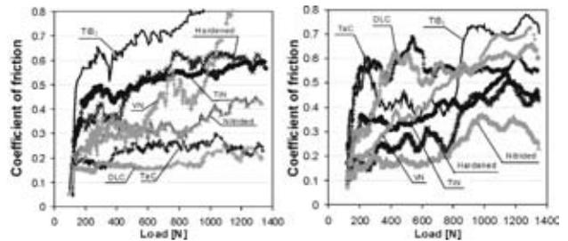
**Figure 2:** Galling properties of surface engineered VANADIS 6 steel against (a) stainless steel and (b) aluminium alloy
