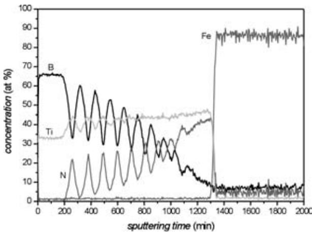
Figure 1: AES sputter depth profile of the  $\text{TiB}_2/\text{Ti(N-B)}/\text{TiN}$
