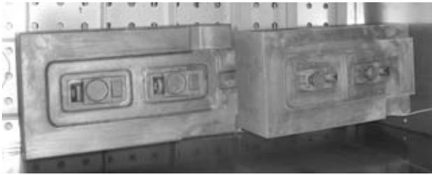
**Figure 2:** A pair of forging dies made of WNL steel processed with nitriding and next cryogenic treatment
