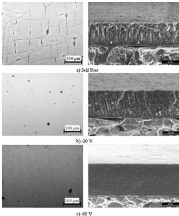
**Figure 2:** SEM images of coating by using different bias voltage: surface (left) cross section (right)
