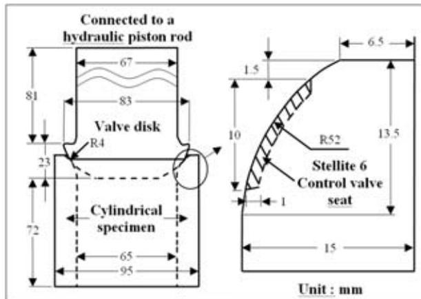
**Figure 1:** Schematic diagram of the impact wear test
