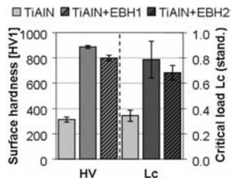
Figure 3: Improvement of surface hardness HV 1 and critical load (standardized values) of TiAlN coatings on C45 (H+T) basic material by subsequent EB hardening
