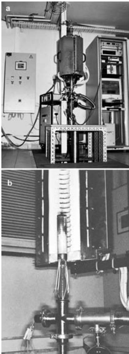
Figure 1: Laboratory device (a) and measurement cell (b) for "in-situ" electrical resistance measurements
