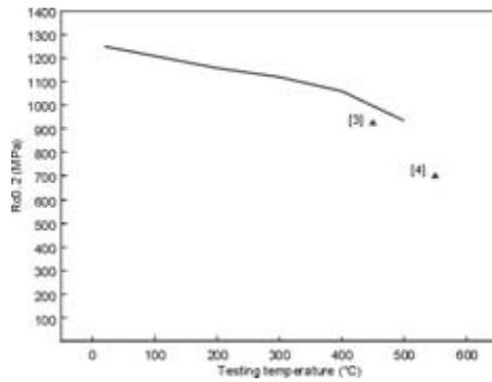
Figure 2: Compressive yield strength at elevated temperatures
