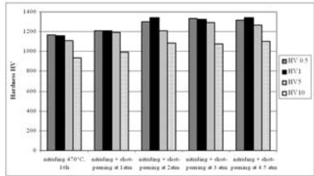
Figure 3: Surface hardness HV0.5, HV1, HV5, HV10 for nitrided layers and surface layers after duplex treatment /nitriding+shot-peening/
