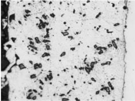
**Figure 1:** Microstructure of Al<sub>12</sub>Si/50SiC<sub>8</sub> composite coating
