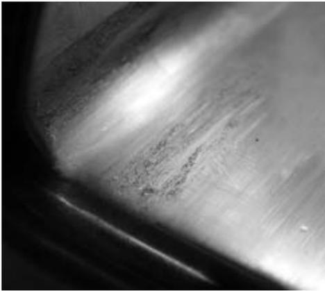
**Figure 2:** Uncoated tool corner area after 100 pieces
