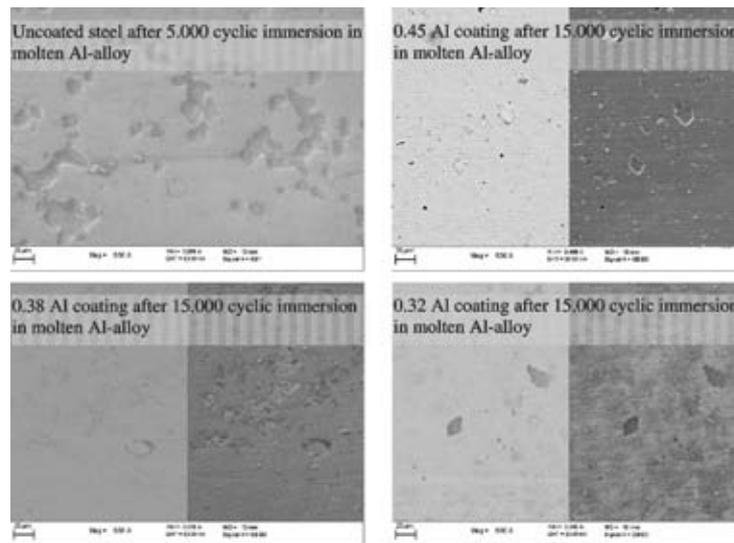
Figure 1: SEM observation of uncoated and coated surface subjected to cyclic immersion in molten aluminium alloy.
