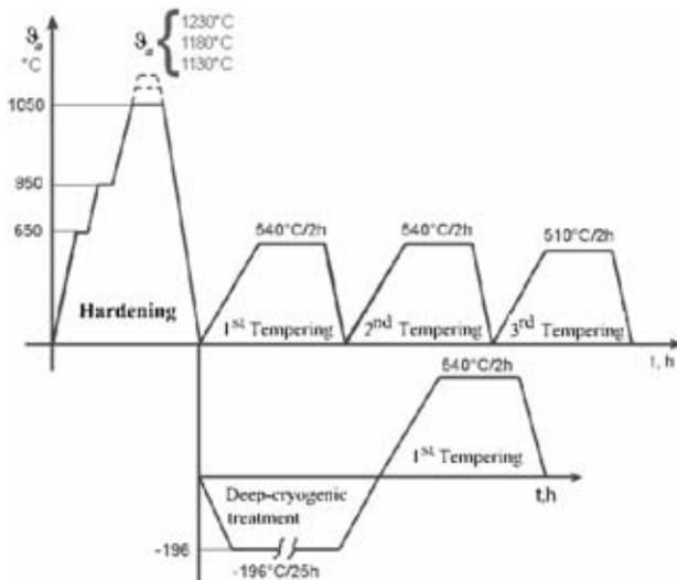
**Figure 1.** Graphical presentation of heat treatment of PM S390 MC high speed steel test samples
