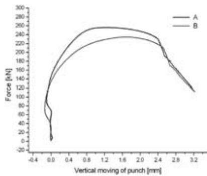
**Figure 3:** Force as function of vertical moving of punch through sheet metal; A – solution annealed alloy Inconel 718 at temperature 960°C, B – solution annealed alloy Inconel 718 at temperature 1050°C
