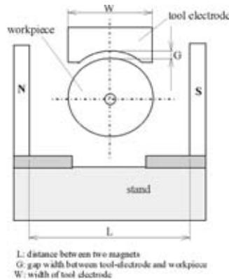
**Figure 2:** Schematics and configuration of the magnetic-assistance system, tool electrode and workpiece
