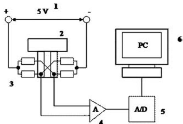
**Figure 1:** Measuring system; 1 – source of electricity, 2 – punch, 3 – strain gauges connected in full Wheatston bridge, 4 – amplifier, 5 – converter of impulse, 6 – personal computer.
