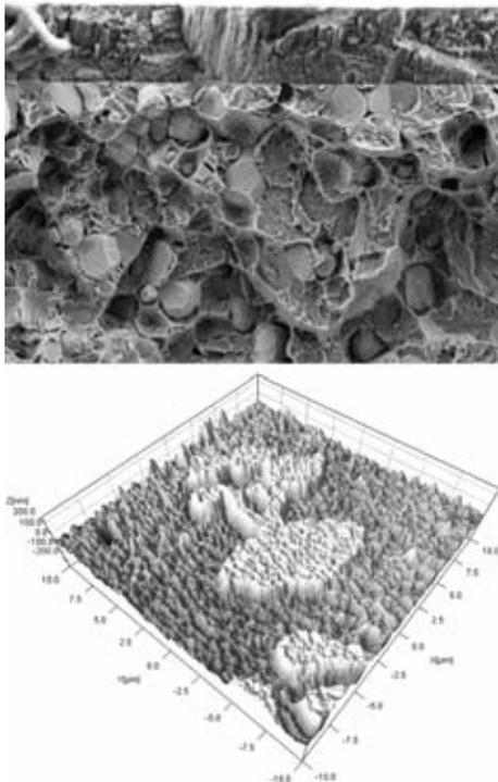
**Figure 1:** Fractured cross-section of AlTiN coating on powder metallurgy cold work tool steel substrates ASP30 (left) and surface topography of D2 cold work tool steel after deposition of AlTiN hard coating (right).
