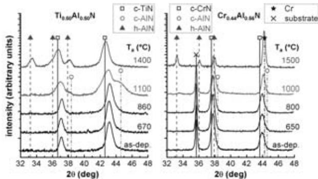
**Figure 1:** X-ray diffraction patterns of  $Ti_{0.50}Al_{0.50}N$  and  $Cr_{0.44}Al_{0.56}N$  after annealing at temperatures  $T_a$
