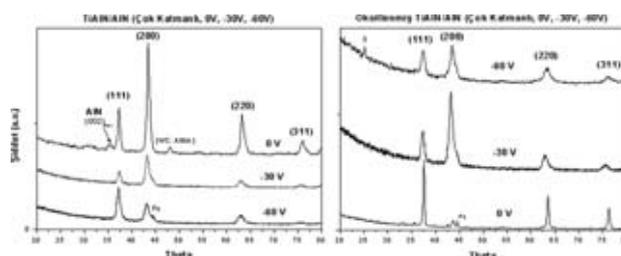
**Figure 1:** Multilayer TiAlN coatings XRD analysis versus different bias voltage: original (left), oxidised (right)
