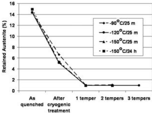
**Figure 1:** The effect of deep cold treatment on retained austenite
