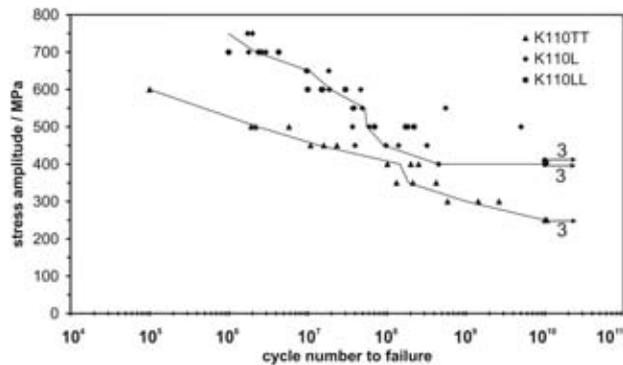
Figure 1: S-N data of AISI D2 type wrought cold work tool steel.
