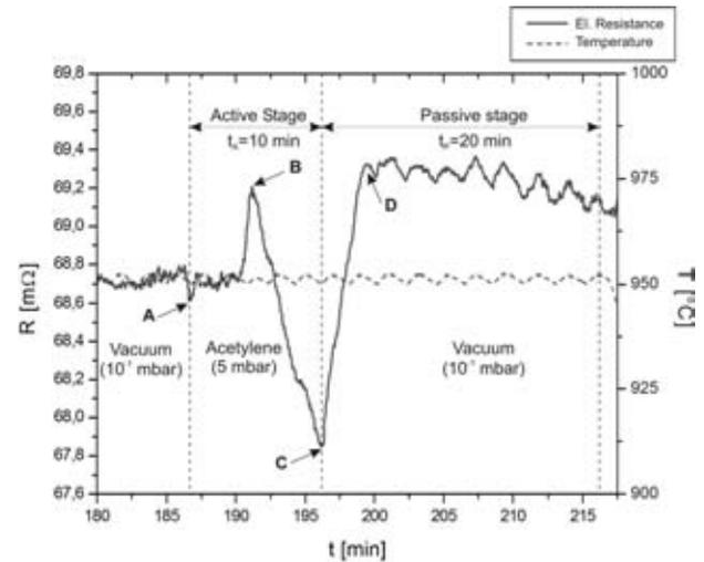
Figure 2: In-situ measurement of electrical resistance changes during vacuum carburizing of the pure iron at T=950°C
