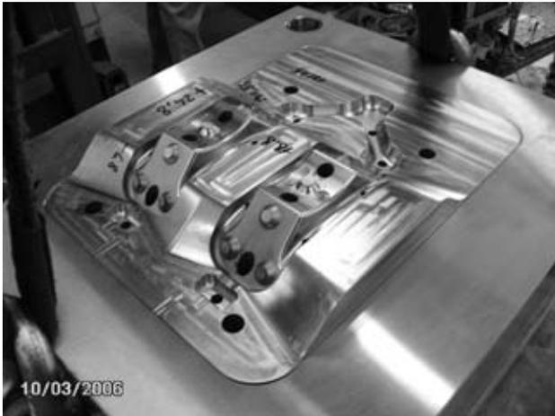
Figure 3: Aluminium pressure die-casting mould
