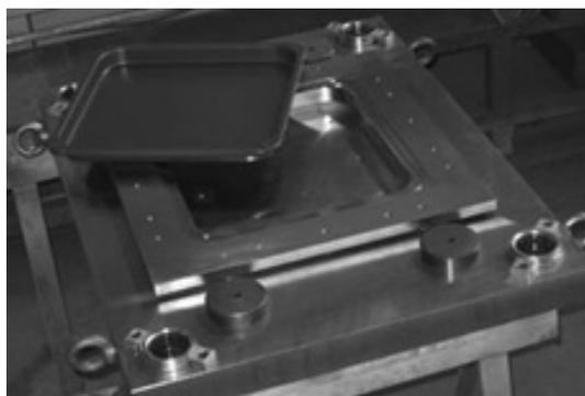
**Figure 1:** Tool for Baking Tray
