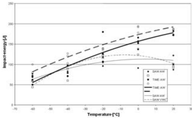
Figure 3: Impact toughness of multipass welds
