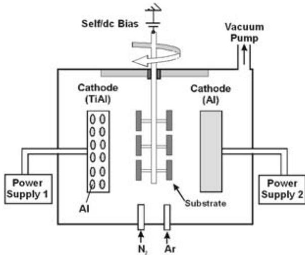
Figure 1: Schematic representation of magnetron sputtering system
