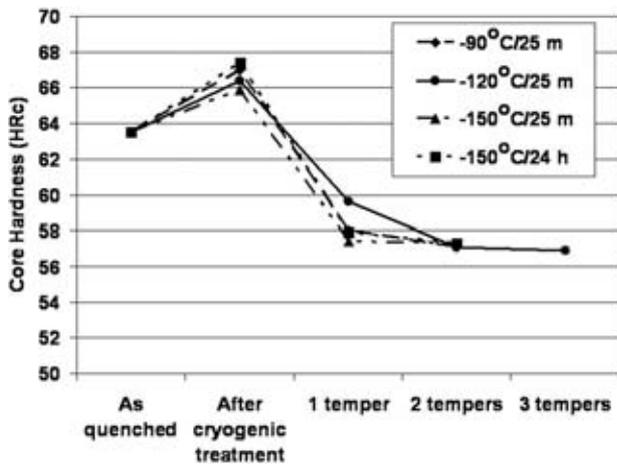
**Figure 2:** The effect of deep cold treatment on hardness
