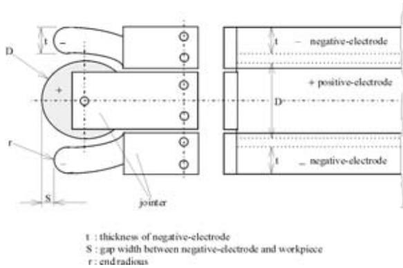
Figure 2: Geometry of electrode
