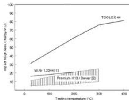
**Figure 1:** Charpy-V impact toughness in regular grades and in TOOLOX 44
