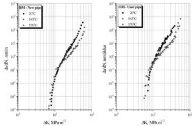
**Figure 1:** Log-log diagram  $da/dN$  –  $\Delta K$  for specimens BM [1]
