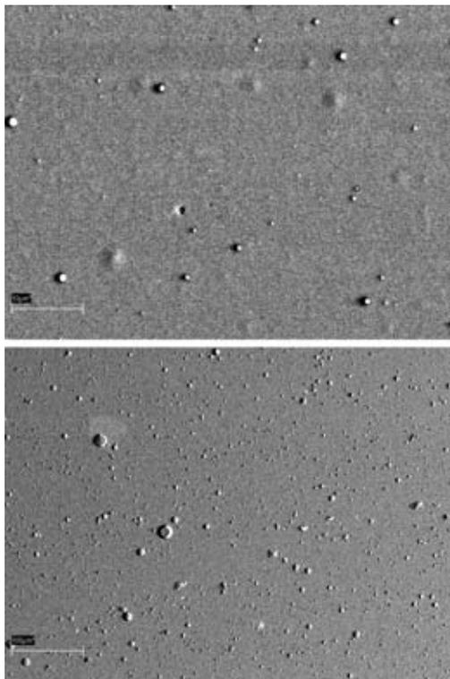
**Figure 1:** The structure of polishing and nitriding X37CrMoV5-1 steel after ion etching: a) Cr ions (marker – 10 μm), b) Ti ions (marker – 10 μm)
