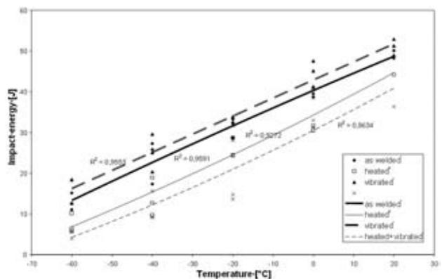
Figure 1: Impact toughness of welds
