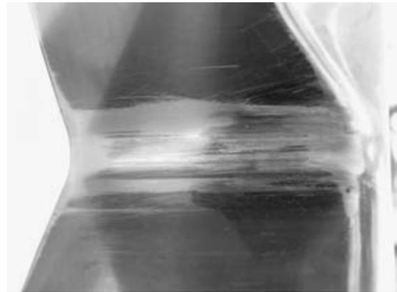
**Figure 3:** TiCN coated tool corner area after 53.000 pieces
