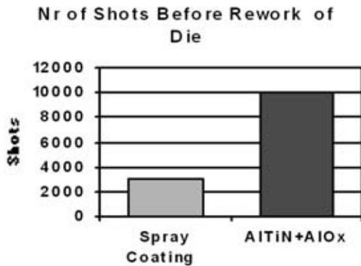
**Figure 2:** Aluminum die casting results /Diesel Injection pump housing
