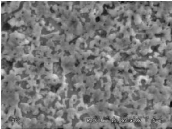
Figure 1: Surface morphology of nitrided layer produced at 470°C, for 16h
