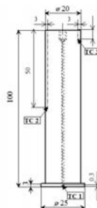
Figure 1: Modified Lohrmann's test specimen
