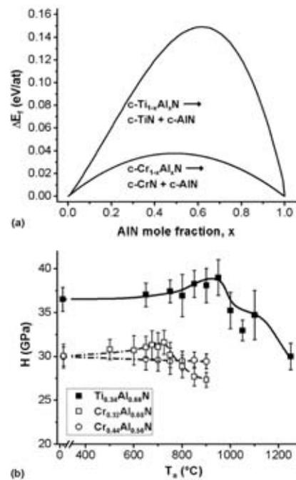
**Figure 2:** (a) Energy of formation difference ( $\Delta E_f$ ) for the separation of  $c-Ti_{1-x}Al_xN$  into  $c-TiN$  and  $c-AlN$  and the separation of  $c-Cr_{1-x}Al_xN$  into  $c-CrN$  and  $c-AlN$  as a function of AlN mole fraction. (b) Hardness ( $H$ ) of  $Ti_{0.34}Al_{0.66}N$ ,  $Cr_{0.32}Al_{0.68}N$  and  $Cr_{0.44}Al_{0.56}N$  as a function of annealing temperature  $T_a$ .
