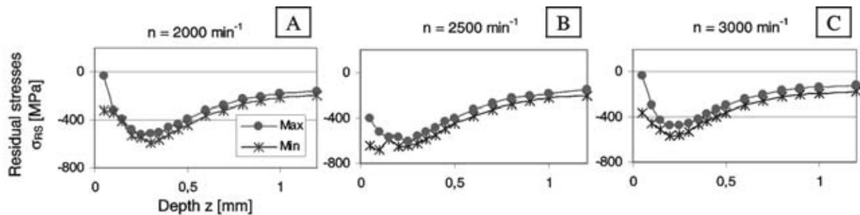
**Figure 1:** Residual-stress profiles of maraging steel after cold deformation of surface layer and after subsequent precipitation hardening at 450°C for 2 hours.
