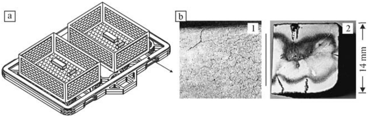
**Figure 1:** The grate from a carburising chamber furnace withdrawn from use: a) schematic diagram, b) surface cracks (1), macrostructure on the wall cross-section (2) with well visible carburised layer, cracks and axial porosity
