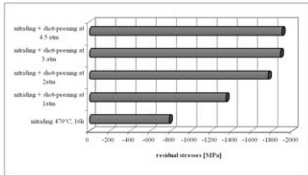
Figure 4: Residual compressive stresses values in the surface layers
