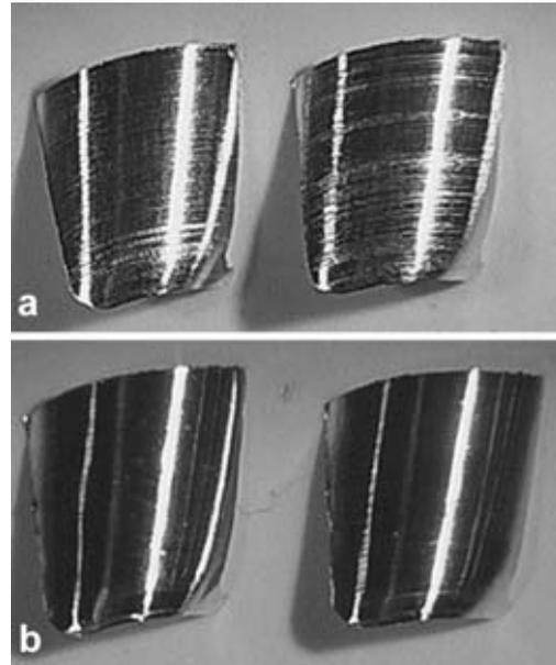
**Figure 3:** Cutting chips from dry Al machining (a – uncoated tool, b – Cr+WC:h+DLC coated tool)
