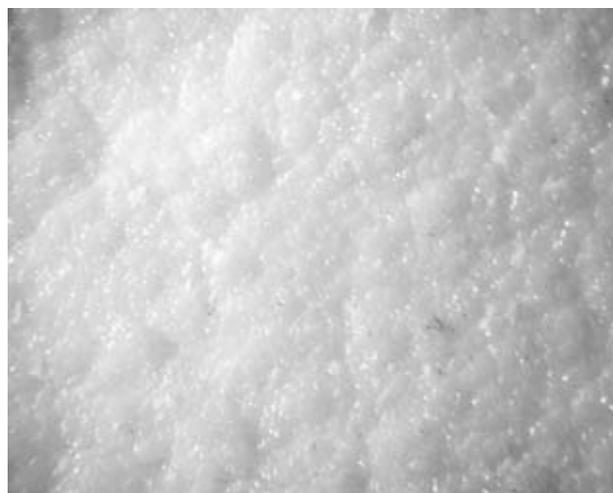
**Figure 1:** The mullite coating stereo microscope figure at 16x
