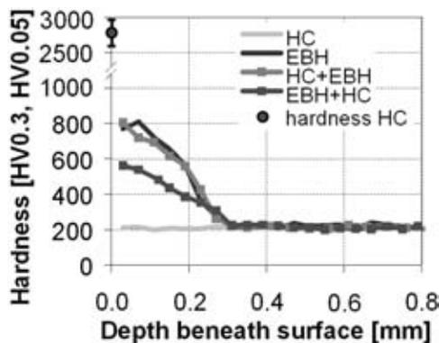
Figure 1: Hardness depth profiles of the combination of HC and EBH
