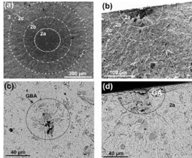
Figure 1: Zones of fatigue crack nucleation and propagation in (a), (c) internal and (b), (d) near-surface failures
