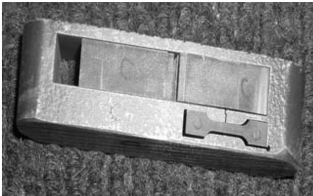
**Figure 1:** Orientation and position of specimens for determination mechanical properties and fracture toughness
