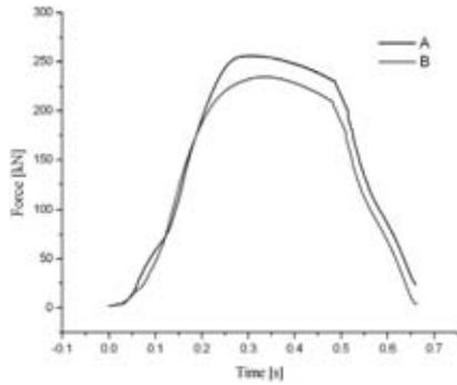
**Figure 2:** Curves for force versus time during process of fineblanking; A – solution annealed alloy Inconel 718 at temperature 960°C, B – solution annealed alloy Inconel 718 at temperature 1050°C
