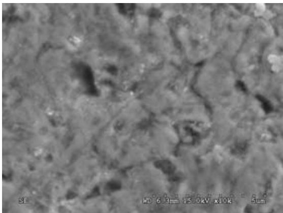
Figure 2: Surface morphology of nitrided layer after shot-peening treatment
