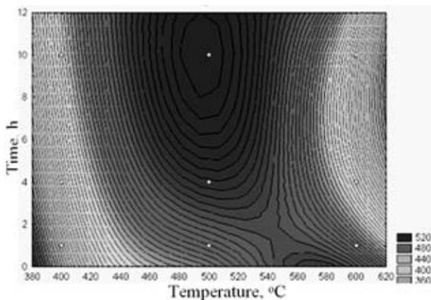
**Figure 1:** Distribution of hardness values HV1 of Maraging 15 10 5 steel depending on factors levels
