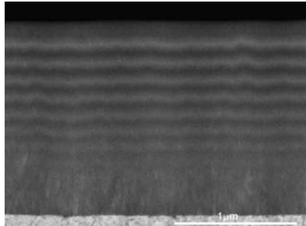
Figure 2: BEI of the nanostructure multilayered coating of a multilayered coated hard sample in cross-section
