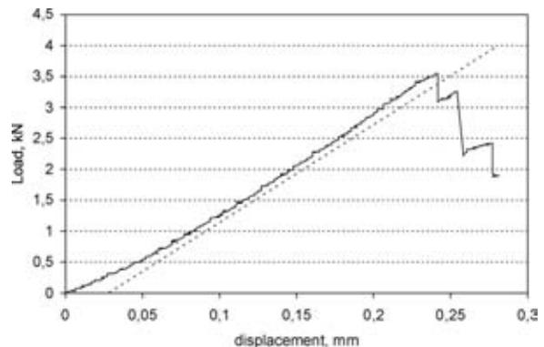
**Figure 2:** Fracture behaviour of single edge bend specimen
