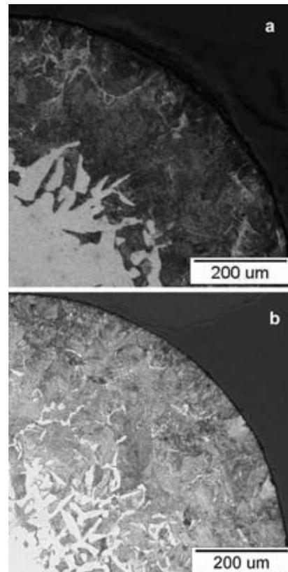
Figure 3: The progress and the morphology of carburized zone after active (a) and passive (b) of the process
