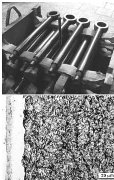
**Figure 1:** View of hydraulics rods oxidation and impregnation after nitriding and microstructure of nitrided 40HM steel (AISI4140)
