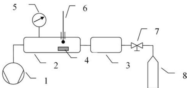
**Figure 1:** The experimental setup for treatment of bacteria with neutral oxygen atoms. 1 – vacuum pump, 2 – experimental chamber, 3 – discharge chamber, 4 – sample, 5 – vacuum gauge, 6 – catalytic probe, 7 – inlet valve, 8 – oxygen flask
