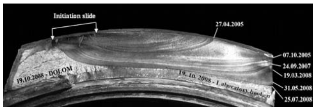
Figure 15: Blade No. 156. Dates, when the crack front reached the line of final blade failure
