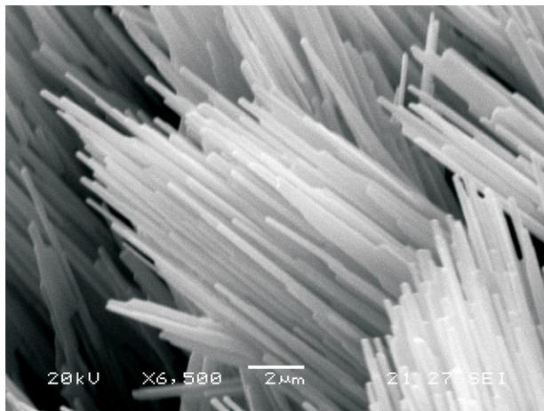
**Figure 2:** Nanowires of niobium pentoxide stretching from the surface of a niobium foil during exposure to an extremely non-equilibrium oxygen plasma with the following parameters: a neutral gas kinetic temperature of about 500 K, an electron temperature of 20 000 K, an ionization fraction of about  $1 \times 10^{-6}$  and a dissociation fraction of about 13 %.
