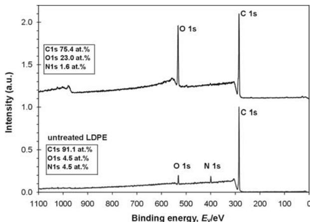
**Figure 4:** The XPS (X-ray photoelectron spectroscopy) survey spectra of untreated and plasma-treated industrial LDPE polymer foil. The oxygen concentration in the surface film of the polymer is increased to 23 % after treatment with plasma with the following parameters: a neutral gas kinetic temperature of about 400 K, an electron temperature of 20 000 K, an ionization fraction of about  $1 \times 10^{-6}$  and a dissociation fraction of about 10 %. The treatment time was 3 s.
