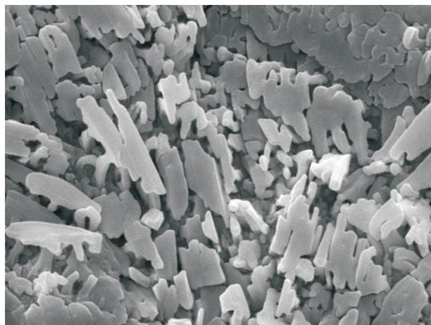
**Figure 3:** Rectangular nanoparticles of niobium pentoxide growing from the surface of niobium foil during exposure to highly non-equilibrium oxygen plasma with the following parameters: a neutral gas kinetic temperature of about 500 K, an electron temperature of 20 000 K, an ionization fraction of about  $8 \times 10^{-7}$  and a dissociation fraction of about 4 %.
