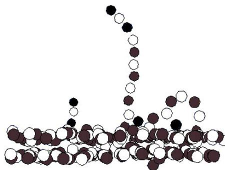
**Figure 1:** The results of a molecular dynamics simulation of the interaction of oxygen atoms added to the surface of nickel foil. The figure shows the formation of NiO chains. Dark and white particles stand for the O and Ni atoms, respectively.
