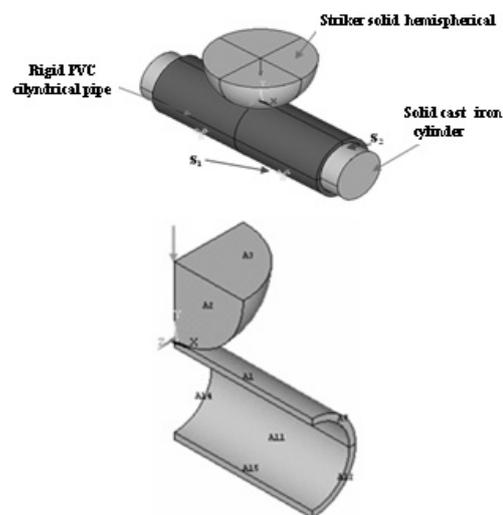
**Figure 5:** Geometric representation of the numerical model: (a) full actual geometry, (b)  $\frac{1}{4}$  of the geometry implemented due to the symmetry of the problem.
