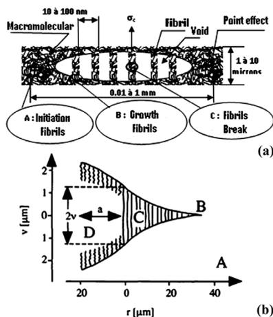
**Figure 1:** (a) Diagram of a craze with cracks characterized by the presence of fibrils <sup>6</sup> (b) Craze region with the result of fissure formation <sup>7</sup>. Zone A represents the region where the glassy polymer is elastically deformed. B, the area where initiation crazing occurs. C propagation or growth of the crazed region. D Rupture of the fibrils leading to the transformation of the craze into a crack of length *a*.
