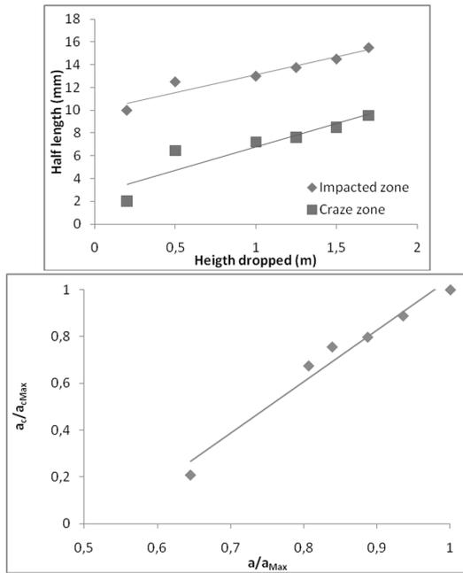
**Figure 9:** (a) Evolution comparison of crazed region "a<sub>c</sub>" and impacted area "a" depending on the level of impact. (b) Evolution of the corresponding non-dimensional "a<sub>c</sub>/a<sub>cMax</sub>" by to "a/a<sub>max</sub>"
