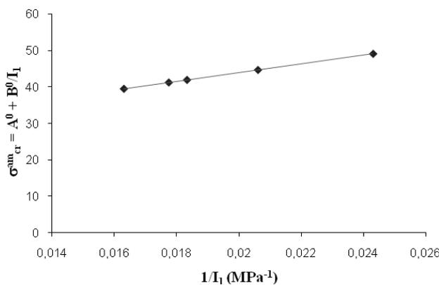
**Figure 6:** A graph of the critical stress of the craze initiation of the Sternstein and Myers criterion  $\sigma_{cr}^{am} = A^0 + B^0/I_1$  around an isovalue contour in the thickness of the pipe.
