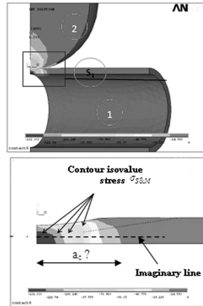
**Figure 7:** Cartograph of stress states  $\sigma_{S\&M} = |\sigma_1 - \sigma_2|$  corresponding to the criterion of Sternstein and Myers. (a)  $1/4$  of the geometry of the pipe, (b) surface  $S_1$  of the thickness of the pipe
