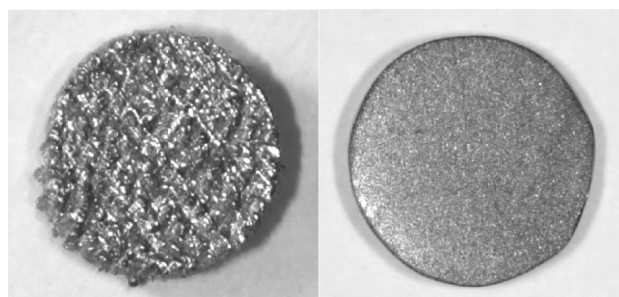
Figure 7: Test samples obtained by SLM (left) and by vacuum casting (right)
