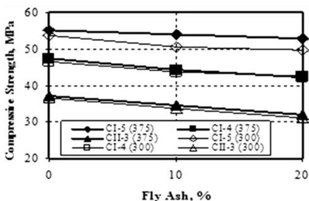
**Figure 3:** Relationship between the compressive strength and the FA amount in 28-day specimens
