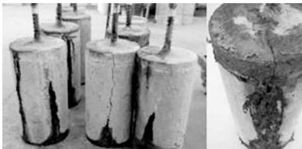
**Figure 6:** Damaged specimens after the impressed voltage test
