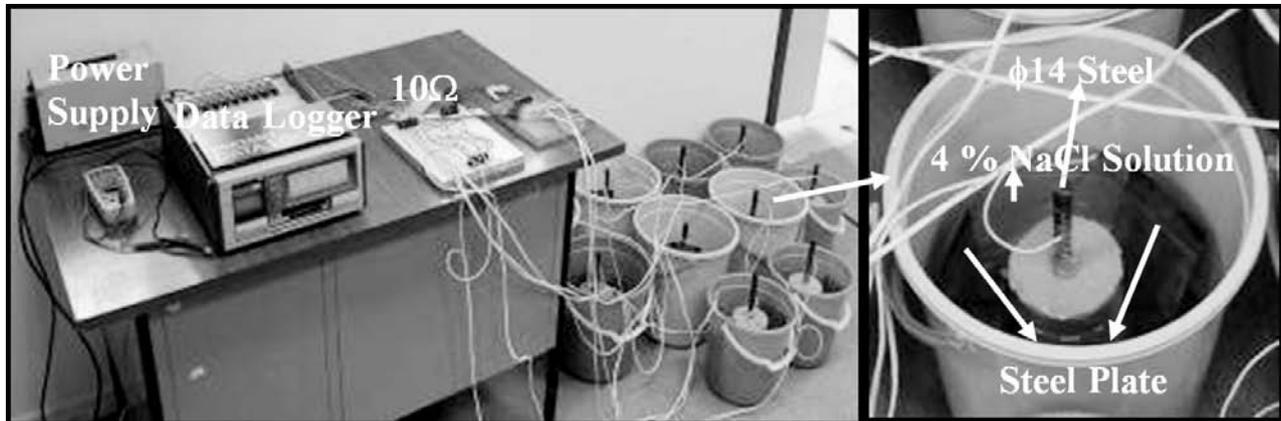
**Figure 2:** Setup for the impressed voltage test
