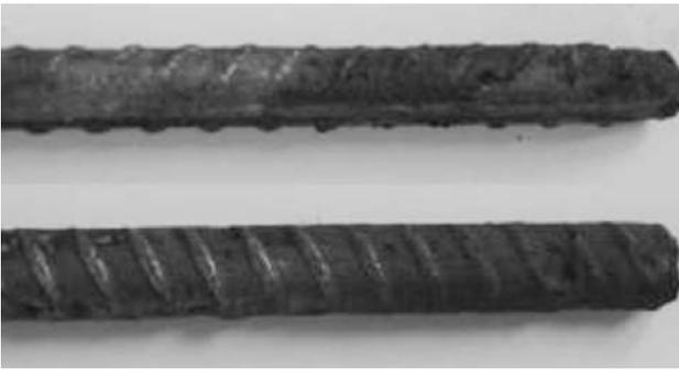
Figure 11: Steel reinforcements cleaned with a Clarke solution
