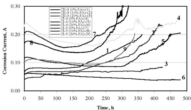
Figure 8: Variation of the corrosion current according to time (a 375-kg/m<sup>3</sup> dosage and 28-day specimens)
