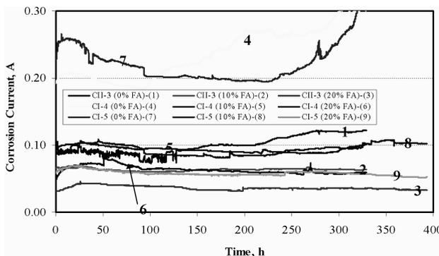
Figure 10: Variation of the corrosion current according to time (a 375-kg/m<sup>3</sup> dosage and 180-day specimens)
