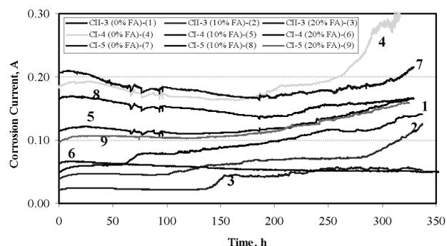
Figure 7: Variation of the corrosion current according to time (a 300-kg/m<sup>3</sup> dosage and 28-day specimens)
