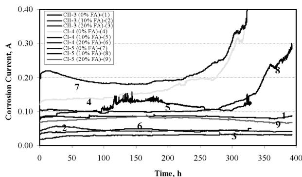
Figure 9: Variation of the corrosion current according to time (a 300-kg/m<sup>3</sup> dosage and 180-day specimens)
