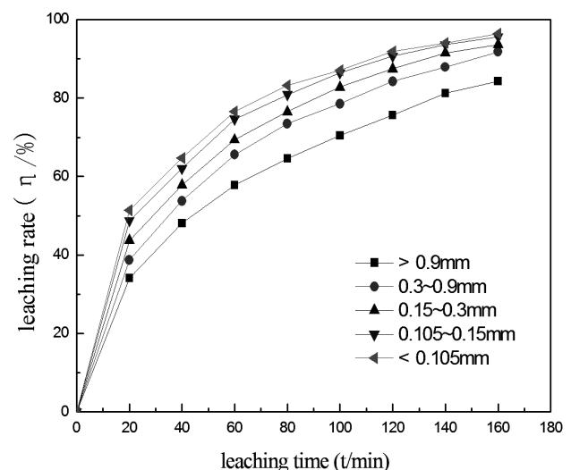
**Figure 4:** Effect of particle size on rare-earth leaching rate
