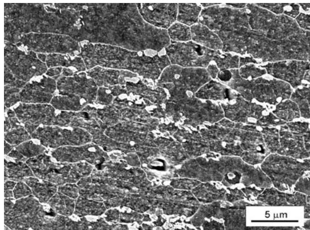
**Figure 5:** 700 °C/10 s – 9-times tension + compression ( $\varphi = 7.2$ ), 30 s pause between deformation cycles
