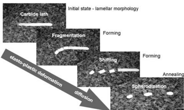
**Figure 1:** Scheme of the newly developed ASR process**Slika 1:** Shematski prikaz novo razvitega postopka
