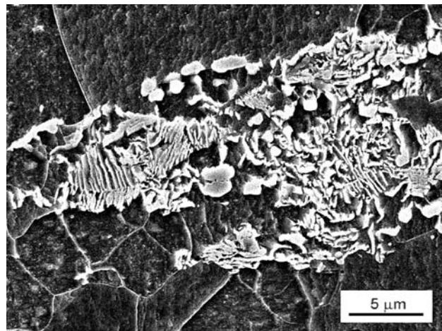
**Figure 6:** 700 °C/10 s – 5-times tension + compression ( $\varphi = 4$ ), 0 s pause between deformation cycles
