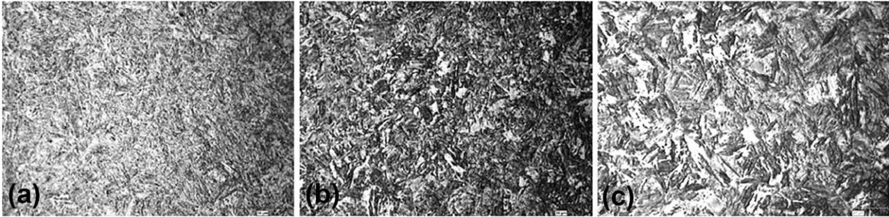
**Figure 2:** Light micrographs of the samples quenched from 850 °C after the austenitization times of: a) 5 min, b) 15 min and c) 30 min
