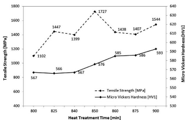
**Figure 5:** Hardness and tensile strength of the samples quenched from (800, 825, 840, 850, 860, 875 and 900) °C after an austenitization time of 15 min
