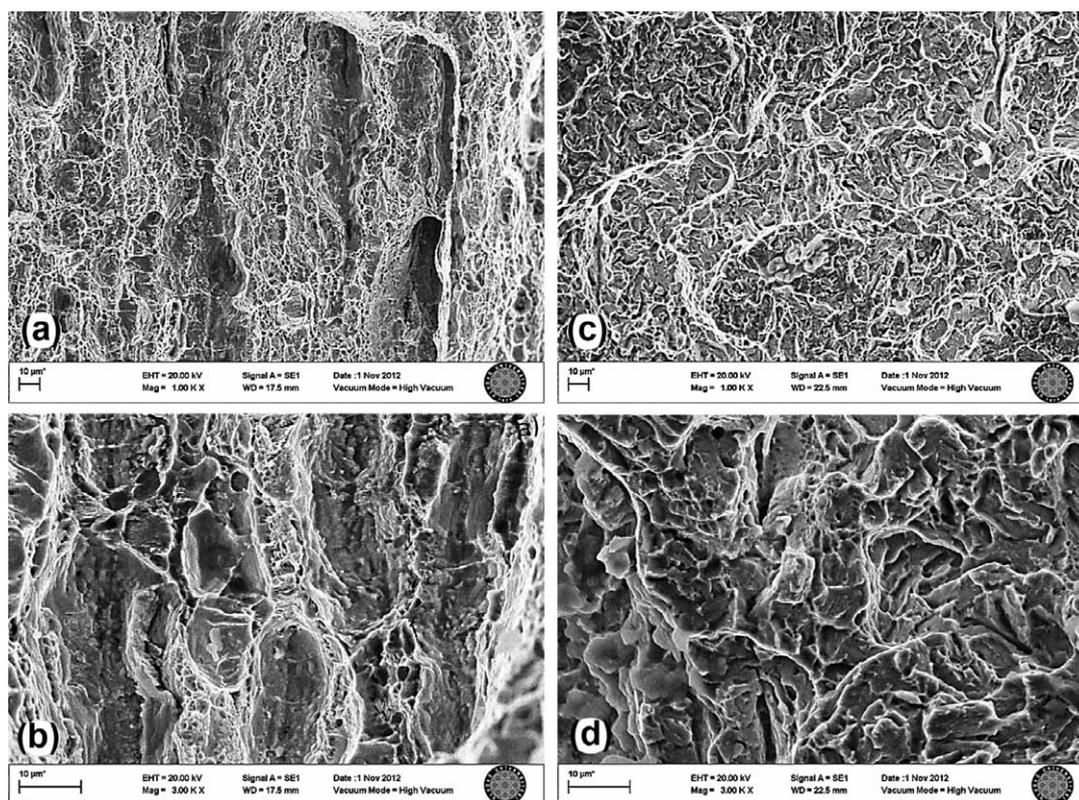
**Figure 6:** SEM images of the fracture surfaces of tensile tested specimens: a) low magnified untreated, b) high magnified untreated, c) low magnified heat treated at 850 °C for 15 min and then quenched and d) high magnified heat treated at 850 °C for 15 min and then quenched
