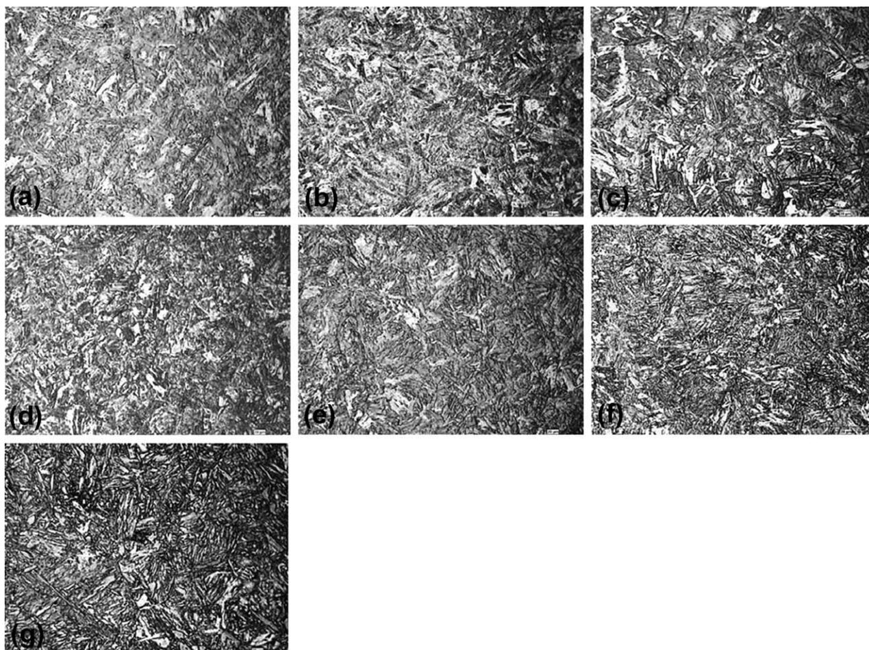
**Figure 4:** Light micrographs of the samples quenched from: a) 800 °C, b) 825 °C, c) 840 °C, d) 850 °C, e) 860 °C, f) 875 °C and g) 900 °C after an austenitization time of 15 min
