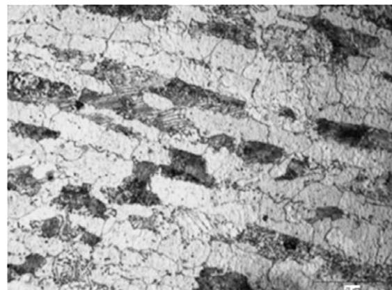
**Figure 1:** Light micrograph of the investigated as-delivered 30MnB5 steel
