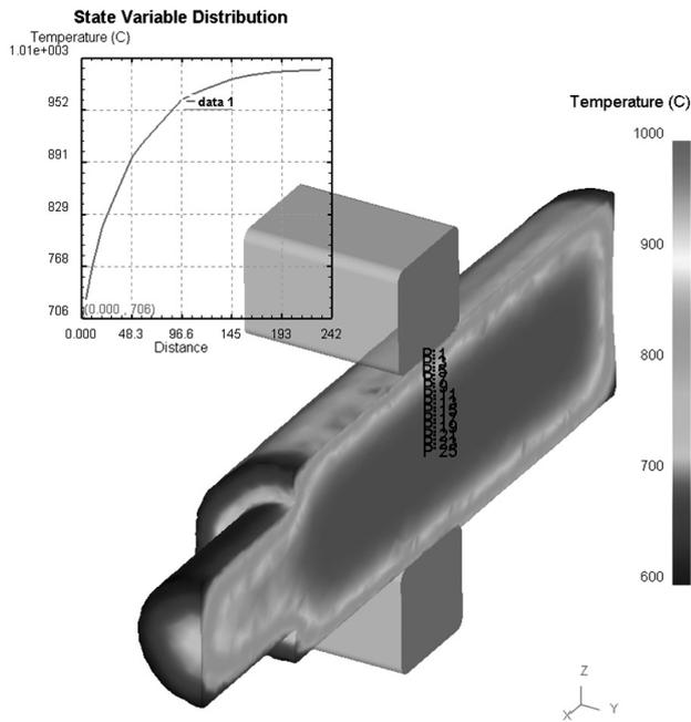
**Figure 1:** Distribution of the temperature for one-step open-die forging – numerical simulation in DEFORM 3D. Diagram in the upper left-hand corner shows the temperature distribution from the surface to the core.
