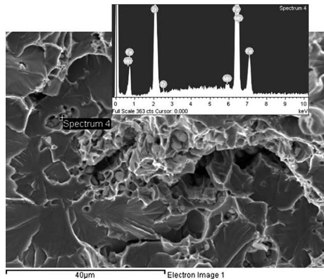
**Figure 8:** ZrCN particles on the fracture surface of heat 15 (SEM)
