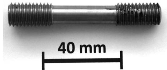
**Figure 3:** Specimen for the physical simulator
