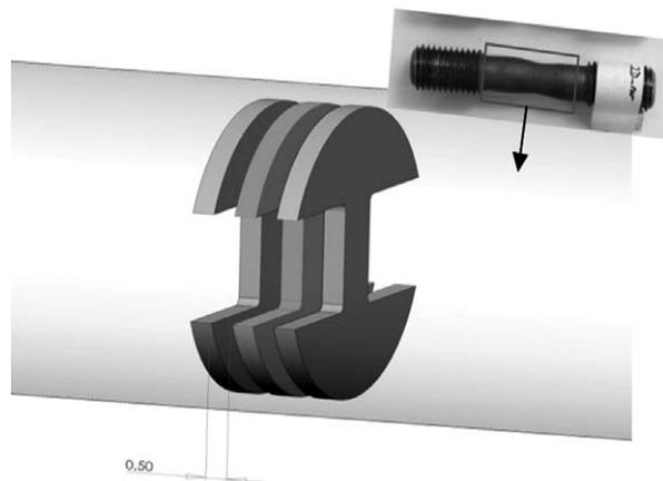
**Figure 6:** Mini-tensile test samples
