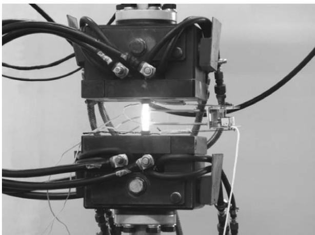
**Figure 2:** Specimen in the physical simulator during thermomechanical processing
