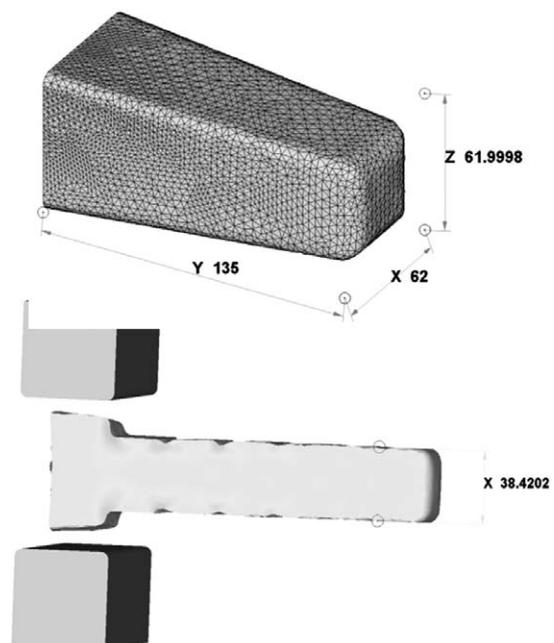
**Figure 9:** Three-dimensional model of an ingot and a numerical simulation of forging in DEFORM 3D
