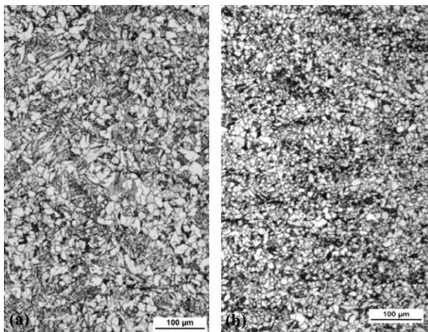
**Figure 7:** Decreased grain size due to a higher deformation: a) specimen Ti1, b) specimen V2
