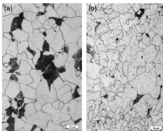
**Figure 10:** Microstructure of the specimens after conventional open-die forging: a) no micro-alloys, b) micro-alloyed with Ti, V and Nb
