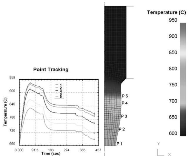
**Figure 4:** Numerical simulation of temperature distribution in the specimen during physical simulation
