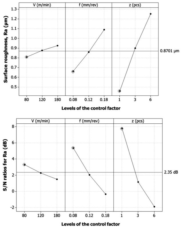
**Figure 4:** Main effects plot of the factors and  $S/N$  graph for the surface roughness
