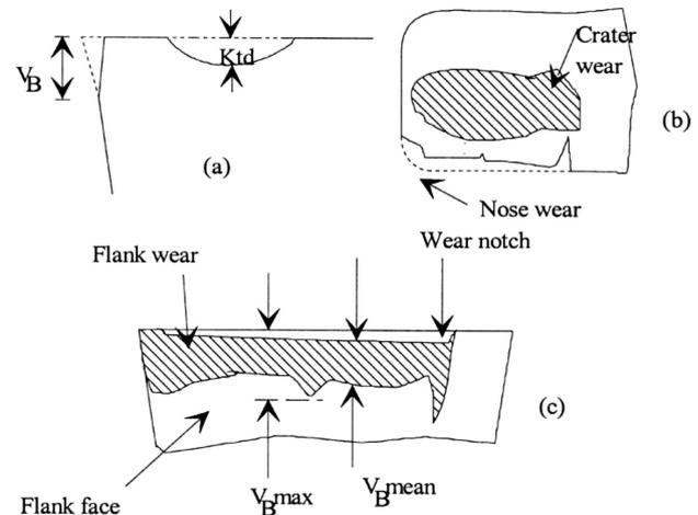
**Figure 3:** Conventional features of tool-wear measurements<sup>17</sup>
