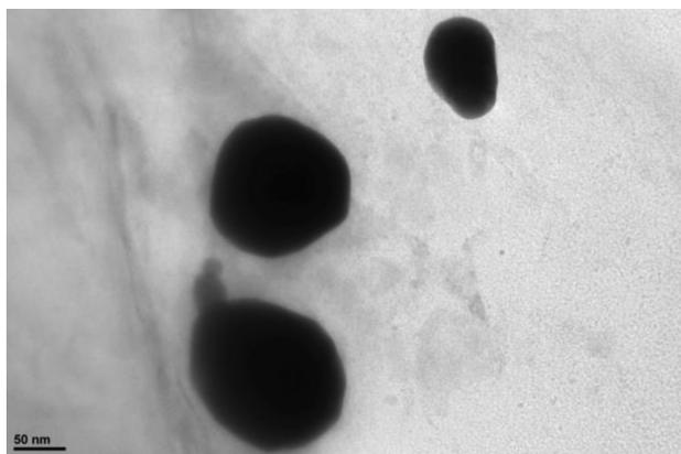
**Figure 8:** Nanoparticles collected on filter paper after evaporation, created with a gold concentration of 1.25 g/L in the precursor solution
