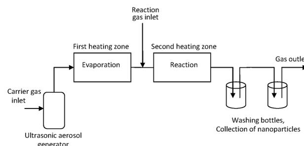
**Figure 3:** Schematic of the modified USP appliance used for experiments
