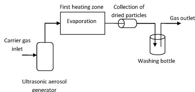
**Figure 5:** Schematic of the device for dried-nanoparticle-collection experiments
