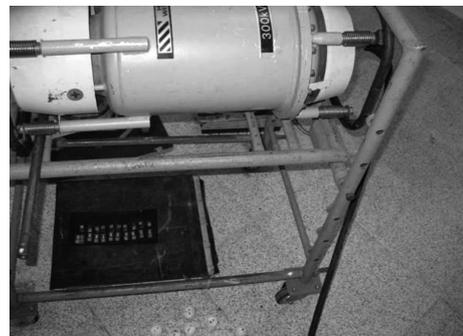
**Figure 6:** Film, penetrometer, stenciling pattern and beam setting
