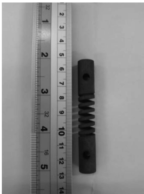
Figure 1: Helicoidal-spring specimen for the stress-change testing
